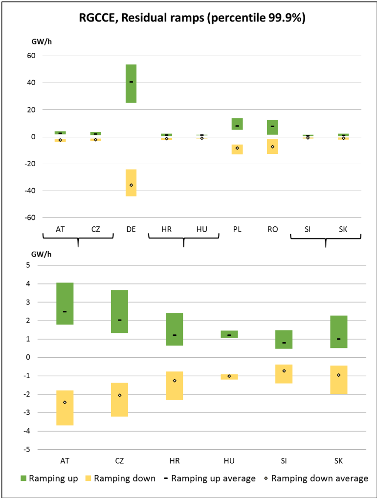
Figure 8-13: Residual ramps in the CCE region in the three studied 2040 scenario with the 2020 grid.
