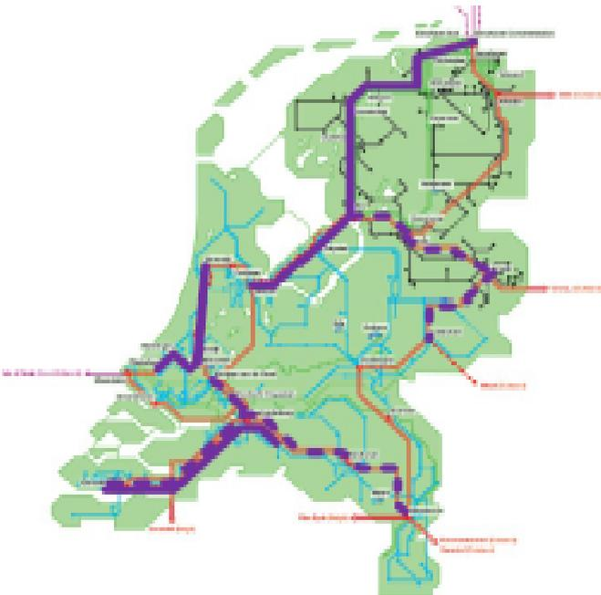
The reinforcements NoordWest380 (to Eemshaven) and ZuidWest380 (to Borssele) are needed to facilitate the bulk (renewable) generation in these areas. Bulk power flows from mainly north to south and east to west, cause overloads in the existing 380kV ring. Further reinforcement is therefore needed to facilitate these flows and also to increase the GTC's between the Germany and the Netherlands, and between Belgium and the Netherlands.
