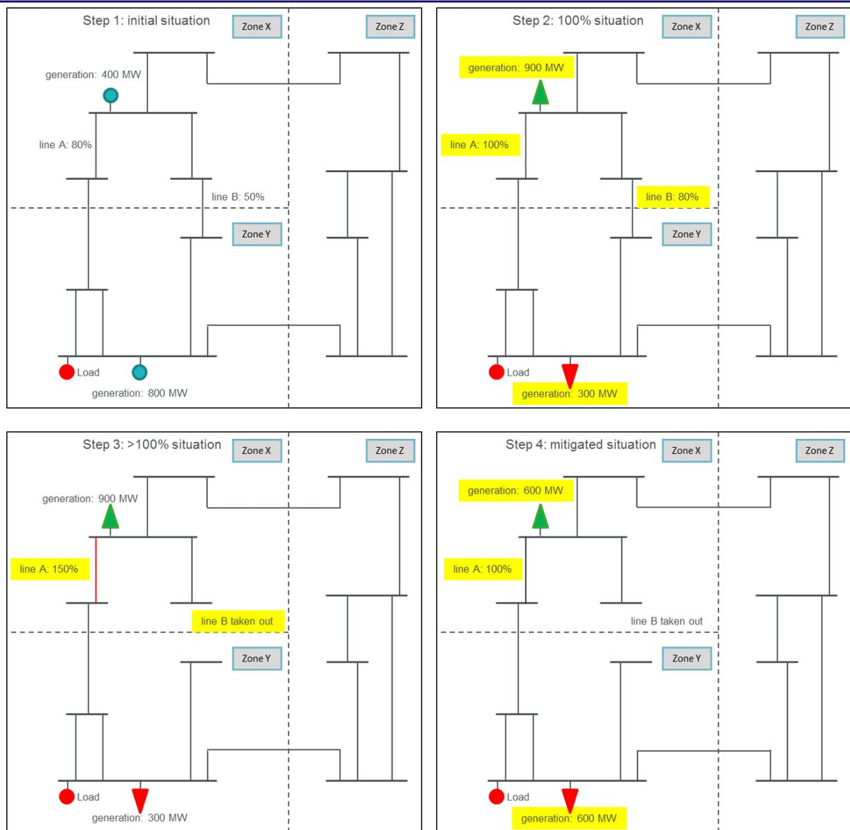
Figure 11: Qualitative example to illustrate the single steps, as described in the example above. It should be noted that the real physical flow will also have a component across the boundary between zones X-Z and Z-Y.
