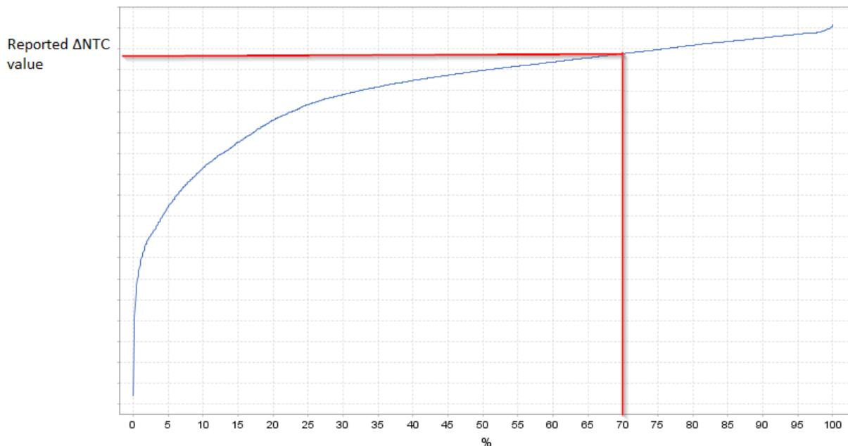
Figure 6: Duration curve of  $\Delta\text{NTC}$  in one direction (blue) with 70<sup>th</sup> percentile (red): the reported  $\Delta\text{NTC}$  at the 70<sup>th</sup> percentile needs to be reached at least 30% of the time –to the right of the red line.
