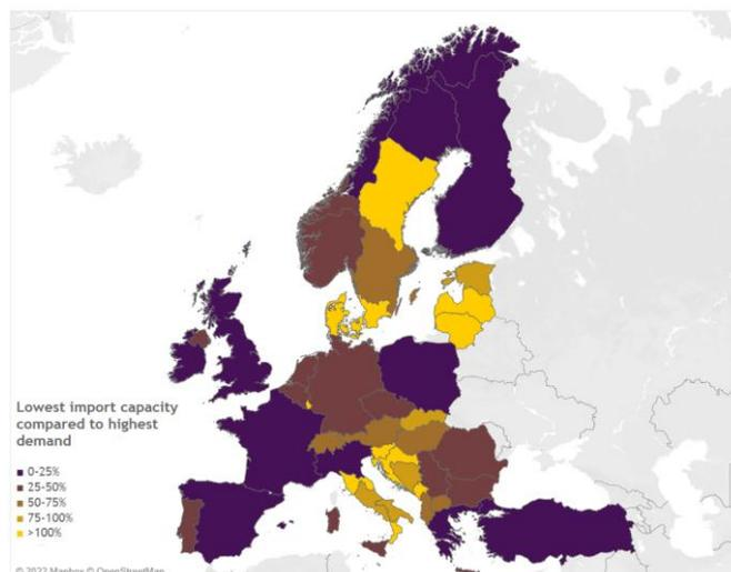
Figure 10: Import capacities per study zone: ratio between lowest import capacity and highest expected demand.
