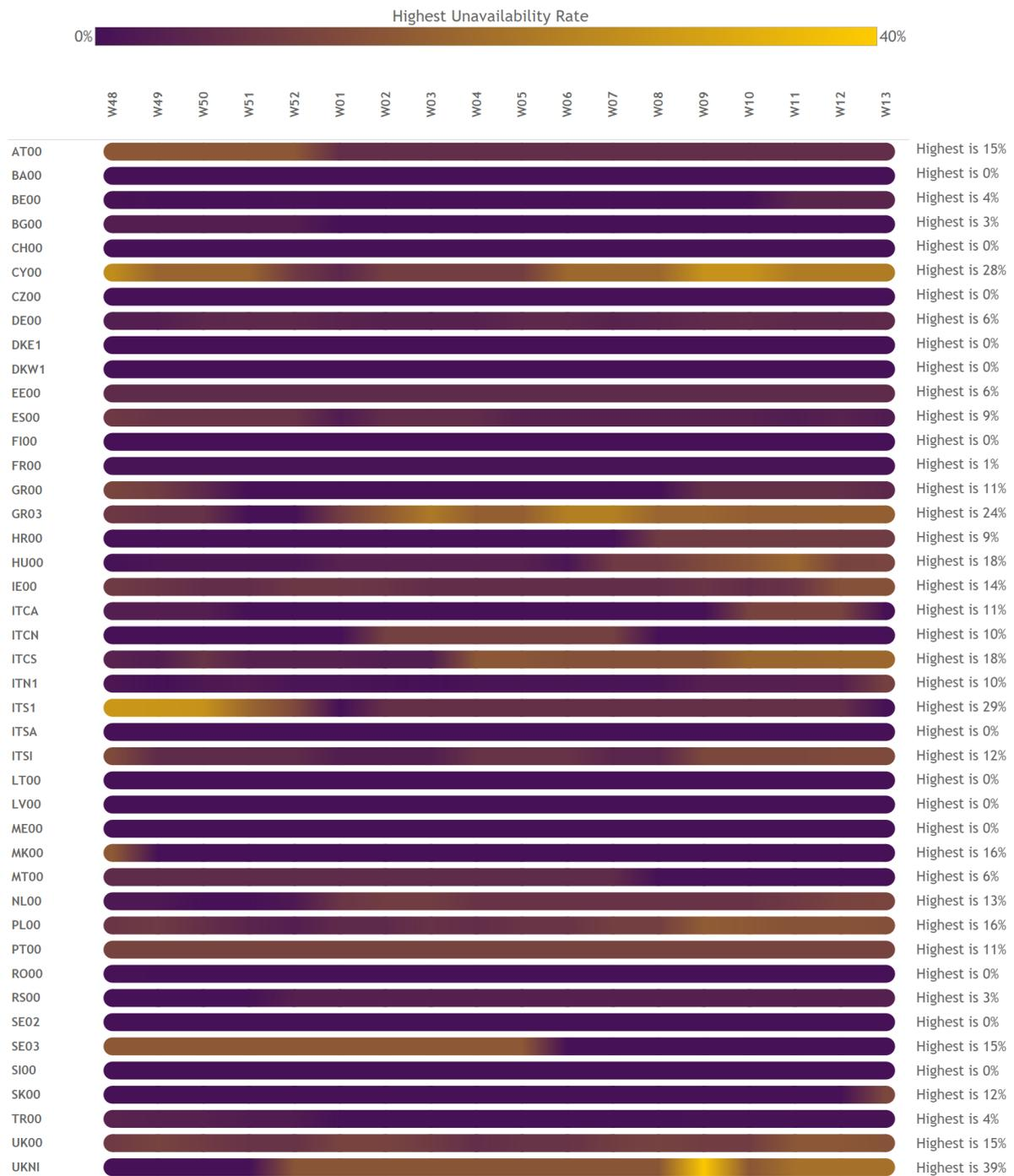
Figure 7: Weekly distribution of thermal planned unavailability relative to thermal NGC
