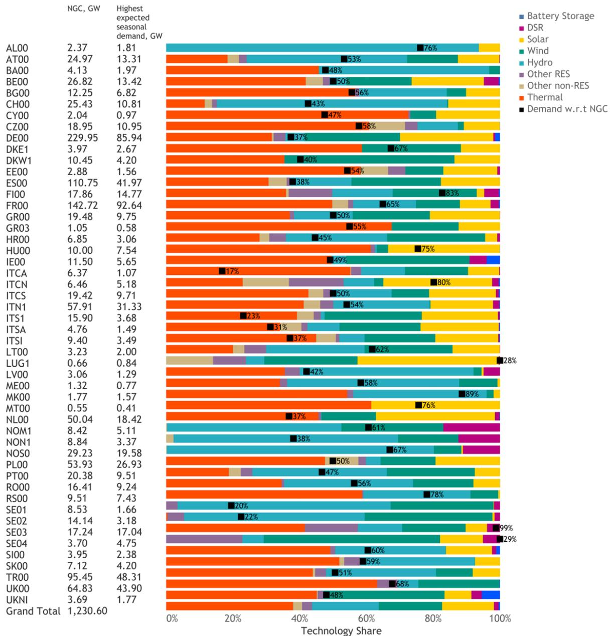
Figure 3: Generation capacity mix at the beginning of winter 2022–2023 per study zone
