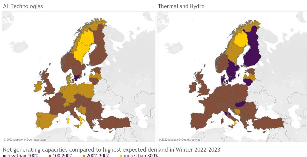
Figure 2: Net generating capacity overview – comparison with highest expected demand
