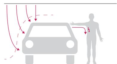
Furthermore, any contact with any lengthy structure that is under the magnetic influence of a live high-voltage line may also result in an electric shock and a contact current. This magnetic induction effect is a well-known safety issue for maintenance tasks of HV lines and it is normally covered by existing safety/security rules. Actions to prevent contact currents and spark discharges are presented in section 4.7.
