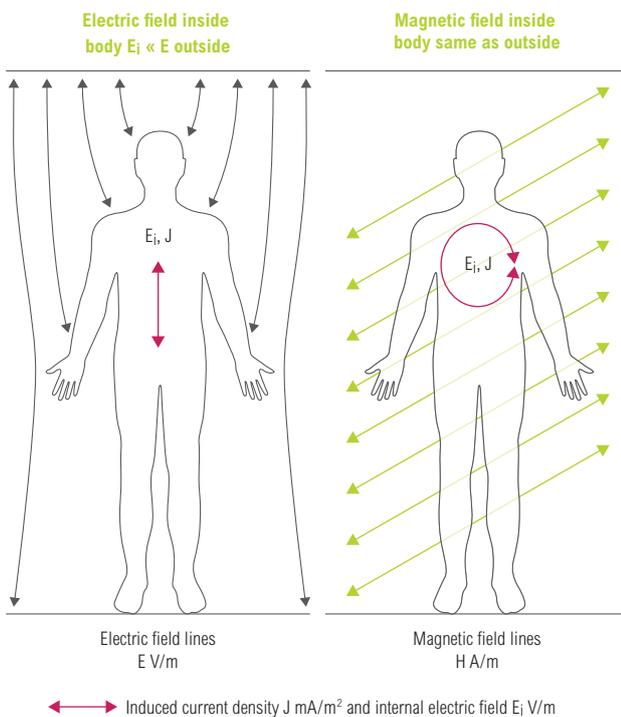
The figures illustrate the induction mechanism for an individual who is exposed to a vertical electric field and to a horizontal magnetic field, such as may occur at ground level under a high-voltage line. In the first case (E-field) a current passes through the body and is then taken away by the ground, in the second case (H-field) the current forms a closed loop in the individual's body.
