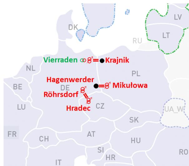
*Reconnection of Krajnik-Vierraden line with PSTs in Vierraden substation plus nearest PSTs in the region. Transitional state until completing project referring PSTs on PL-DE border.*
