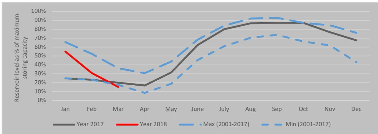
Figure 15: Reservoir levels in Austria.<sup>14</sup>
