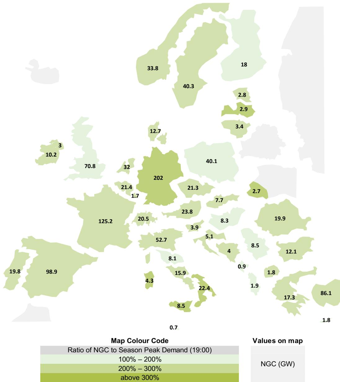
Figure 2: Net generating capacities (in GW) and colour according to its ratio to expected national peak demand in the summer season.
