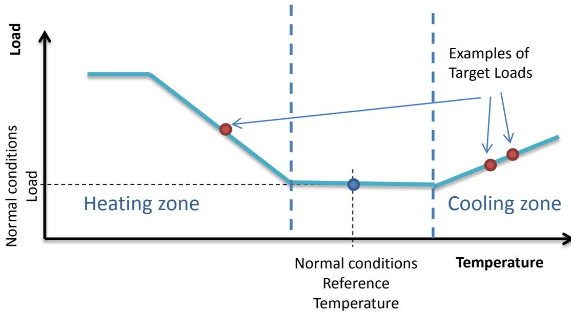
Figure 1 – Load temperature sensitivity
