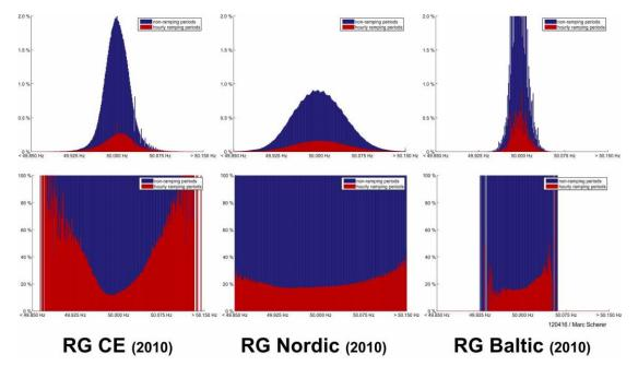
Figure 12: Distribution of Frequency Deviations in CE, Northern Europe (Nordic) and Baltic for 2010 distinguishing all minutes and the minutes around the change of the hour.
