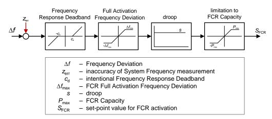
Figure 34: Implications of accuracy requirements – simplified control scheme
