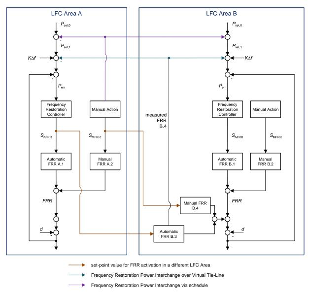
Figure 22: Example for TSO-Provider Activation with Virtual Tie-Lines and schedules
