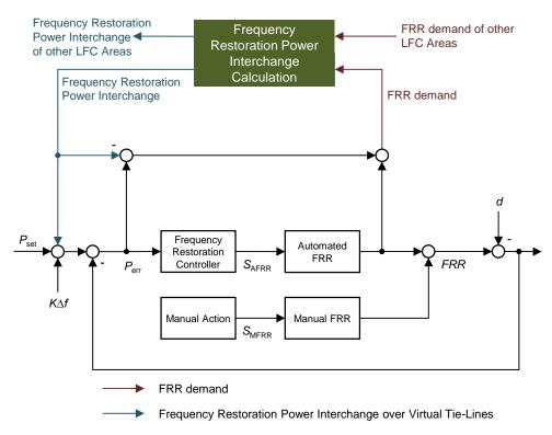
Figure 23: Example for TSO-TSO Activation for automated FRR with Virtual Tie-Lines
