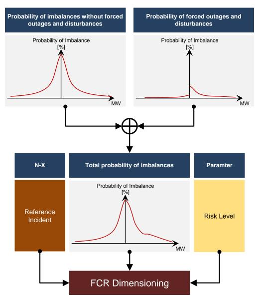
Figure 26: Probabilistic approach for FCR dimensioning
