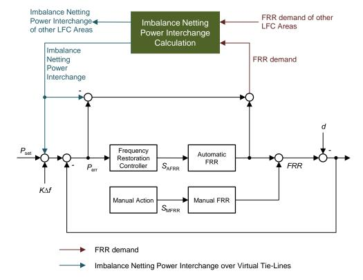
Figure 20: Integration of Imbalance Netting Process into the Frequency Restoration Process
