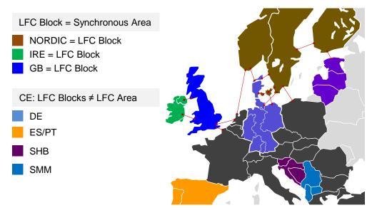
Figure 16: Synchronous Areas, LFC Blocks and LFC Areas
