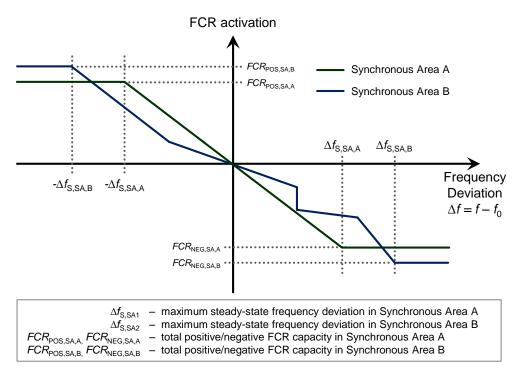
Figure 17: Example for the design of total FCR response in a two Synchronous Areas
