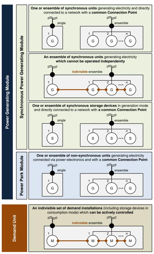
Figure 30: Power Generating Module and Demand Unit
