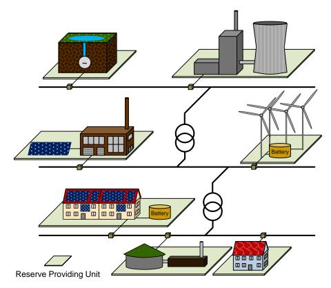
Figure 32: Illustration of possibilities for aggregation within a Reserve Providing Unit
