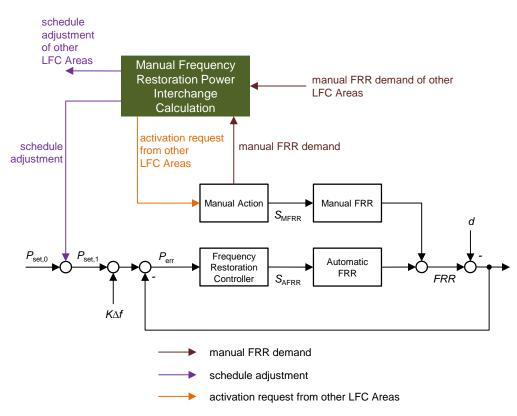
Figure 24: Example for TSO-TSO Activation for manual FRR with schedules
