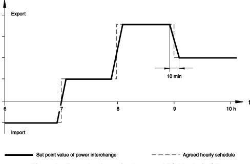
Figure 50: Example of ramping between LFC Blocks in CE
