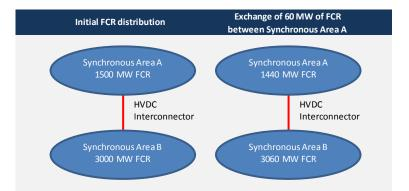
Figure 41: Example for the Exchange of FCR between two Synchronous Areas
