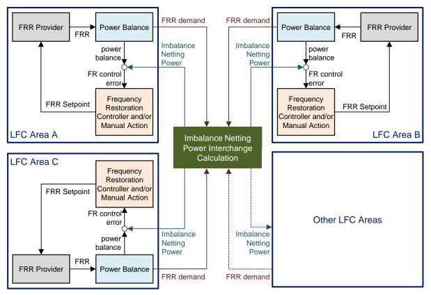
Figure 19: Imbalance Netting Process – basic principle
