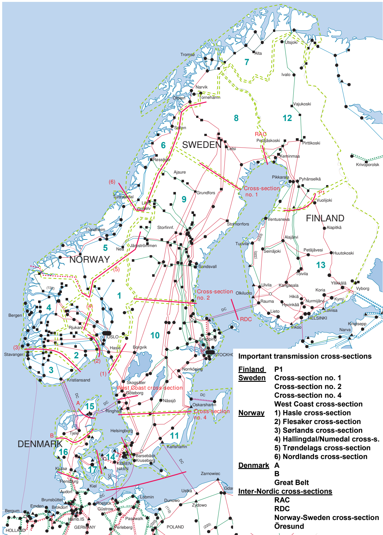
Figure 5 Important transmission cross-sections in the Nordel area shown in relation to the area division (areas 1 – 17) for which power and energy analyses are made.
