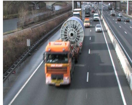
Figure 2: 400kV XLPE drums transported by truck
