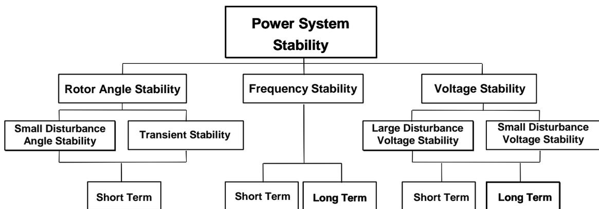
Figure 1: Classification of Power System Stability according to “Definition and classification of power system stability” IEEE/CIGRE Joint Task Force, June 2003
