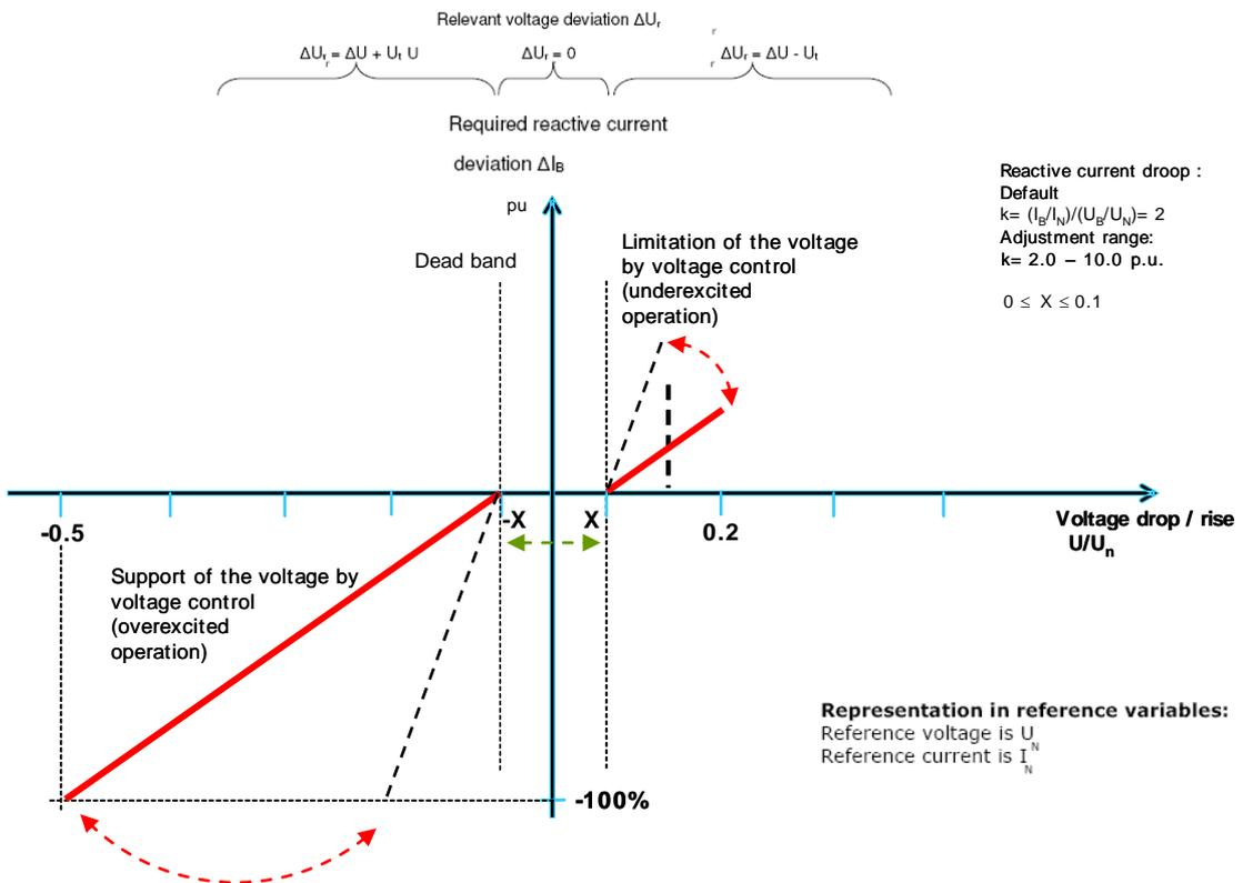
Figure 16 – Principle of voltage support during faults
