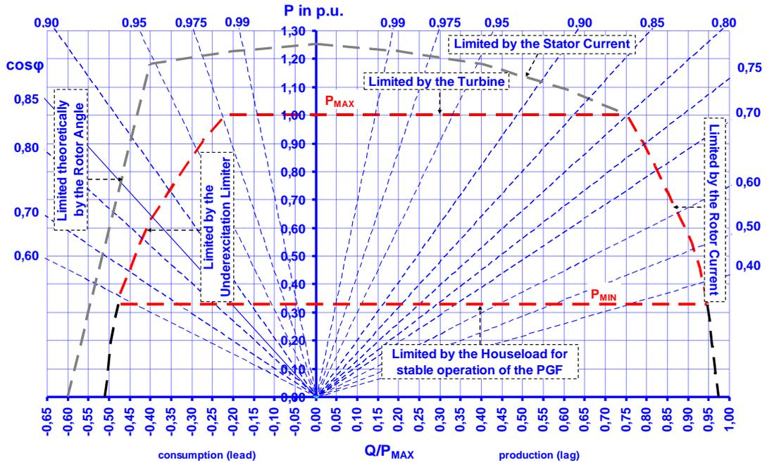
Figure 8 – Typical P-Q-Capability Diagram of a synchronous generator
