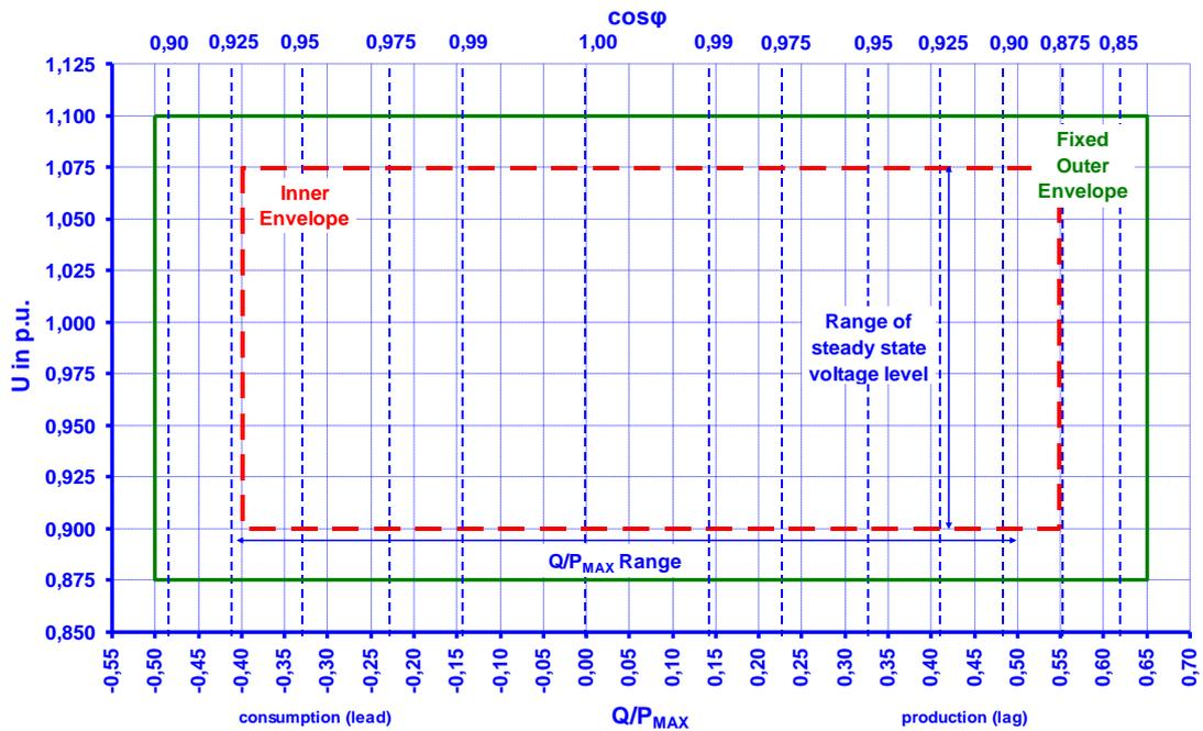
Figure 7 – **Reactive Power** capacity diagram
