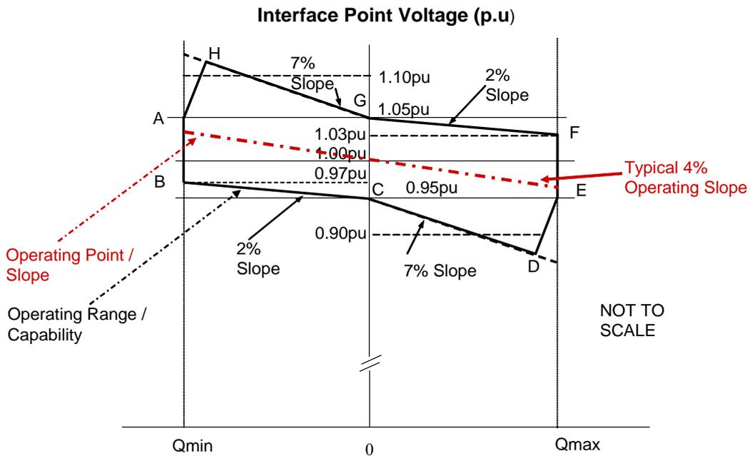
Figure 15 – Steady-state voltage control of **Power Park Modules**
