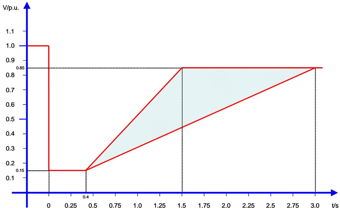
Figure 14 – Voltage-against-time-profile at the **PCC** for **Power Park Modules** connected at voltage levels below 110 kV
