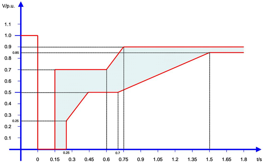
Figure 9 – Boundaries of a voltage-against-time-profile (red lines) at the **PCC** for **Synchronous Generating Units** connected at voltage levels at 110 kV or above
