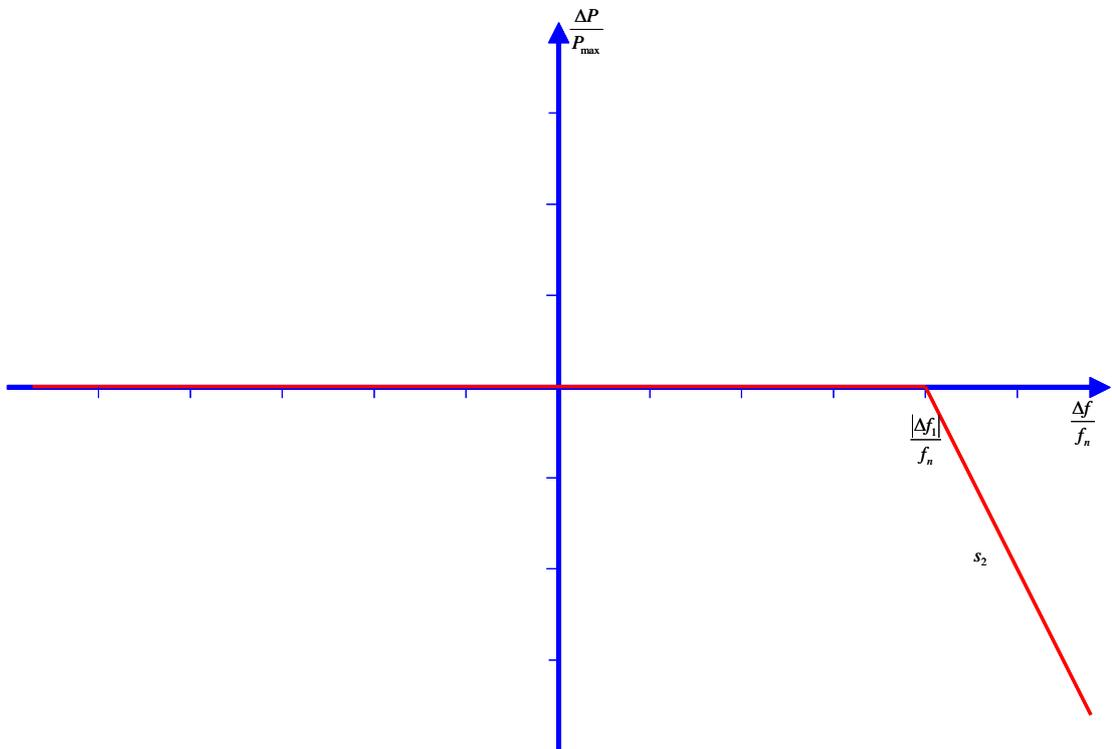
Figure 5: **Active Power Frequency Response** of **Power Generating Units** in limited frequency sensitive mode (overfrequency)
