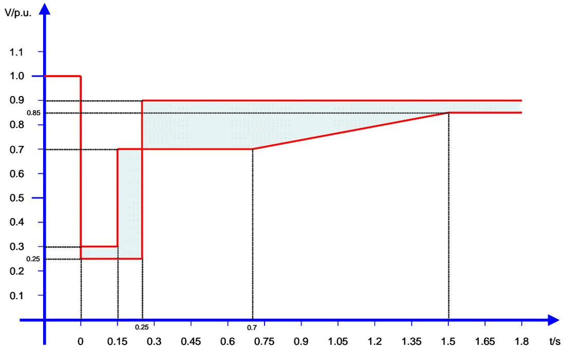
Figure 10 – Boundaries of a voltage-against-time-profile (red lines) at the **PCC** for **Synchronous Generating Units** connected at voltage levels below 110 kV
