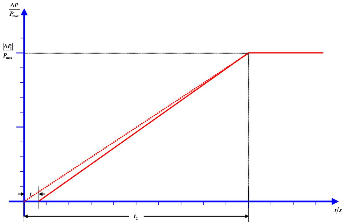
Figure 4: Timeframe for full activation of **Active Power Frequency Response**
