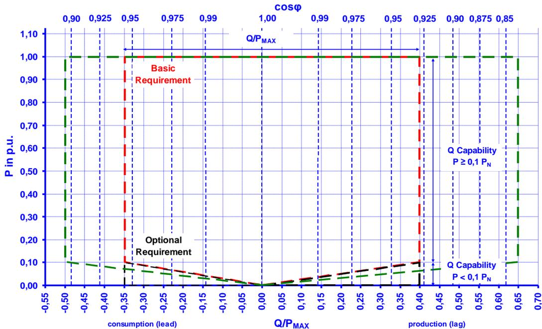
Figure 12 – Typical P-Q-Capability Diagram of a **Power Park Module**
