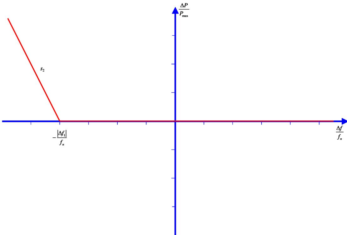
Figure 6: **Active Power Frequency Response** of **Power Generating Units** in limited frequency sensitive mode (underfrequency)
