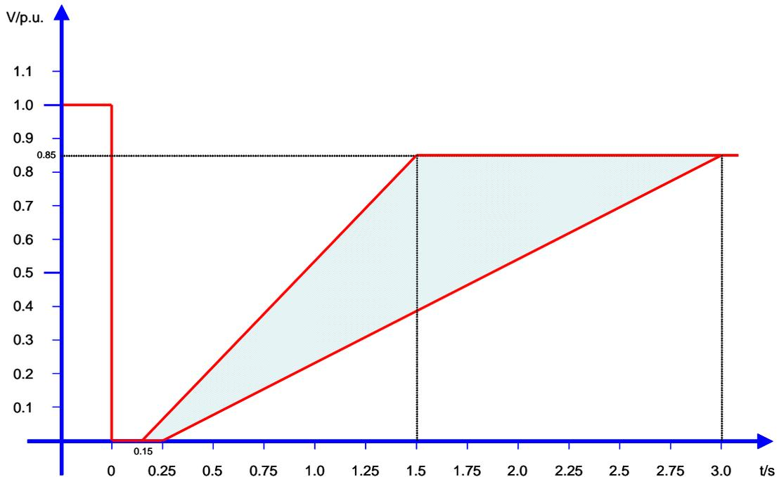
Figure 13 – Boundaries of a voltage-against-time-profile (red lines) at the **PCC** for **Power Park Modules** connected at voltage levels at 110 kV or above
