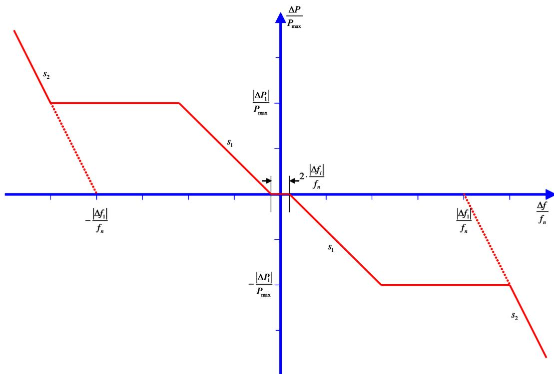
Figure 3: **Active Power Frequency Response of Power Generating Units** in frequency sensitive mode
