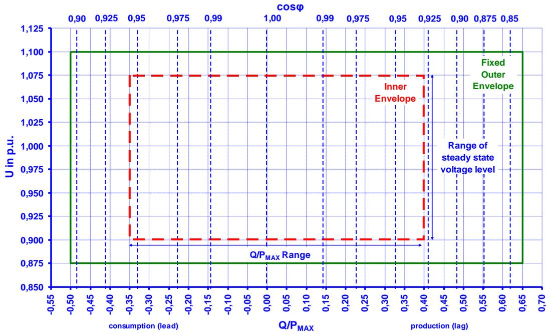
Figure 11 – Reactive Power capacity diagram
