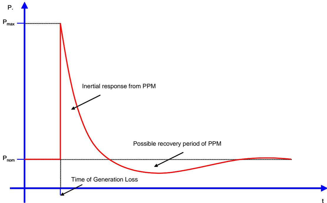
Figure 17: Example of **Active Power** provision by inertia
