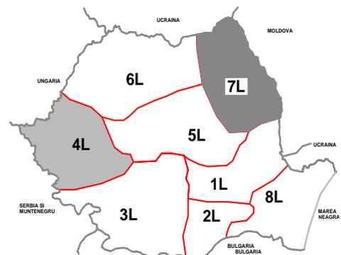
8 Load zones highlighting the load deficit area (4L) and load surplus area (7L)
