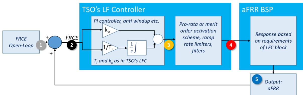
Figure 3: Generic overview of automatic frequency restoration process
