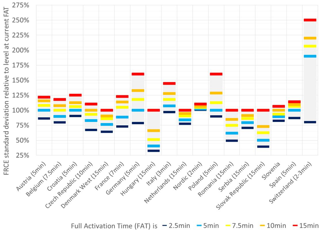
Figure 22: FRCE standard deviation for a change from the existing FAT to a FAT of 2.5, 5, 7.5, 10 and 15 minutes, relative to the situation with a simple merit order activation scheme and the existing FAT (between brackets FAT)<sup>22</sup>
