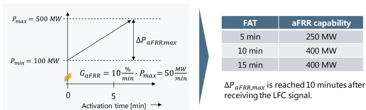
The ramp rate of  $10 \frac{\%}{min}$  leads to possible change in power output of  $50 \frac{MW}{min}$ . This means that FAT of 3 minutes would lead to a theoretical aFRR capability of 150 MW, or with a FAT of 15 minutes to a capability of 400 MW.
