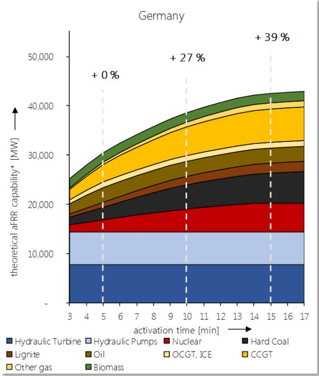
Figure 20: Example of a theoretical aFRR capability diagram for Germany (percentages are the change from current FAT) \* Upward and downward, not symmetric
