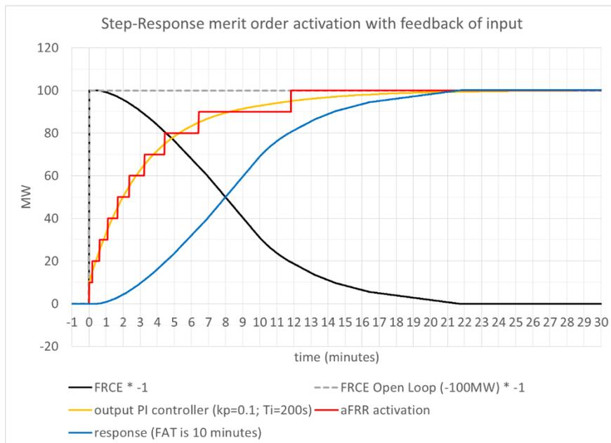
Figure 18: Step response for 100MW step of merit-order activation scheme with a feedback loop (to be compared with Figure 11) <sup>12, 17</sup>.
