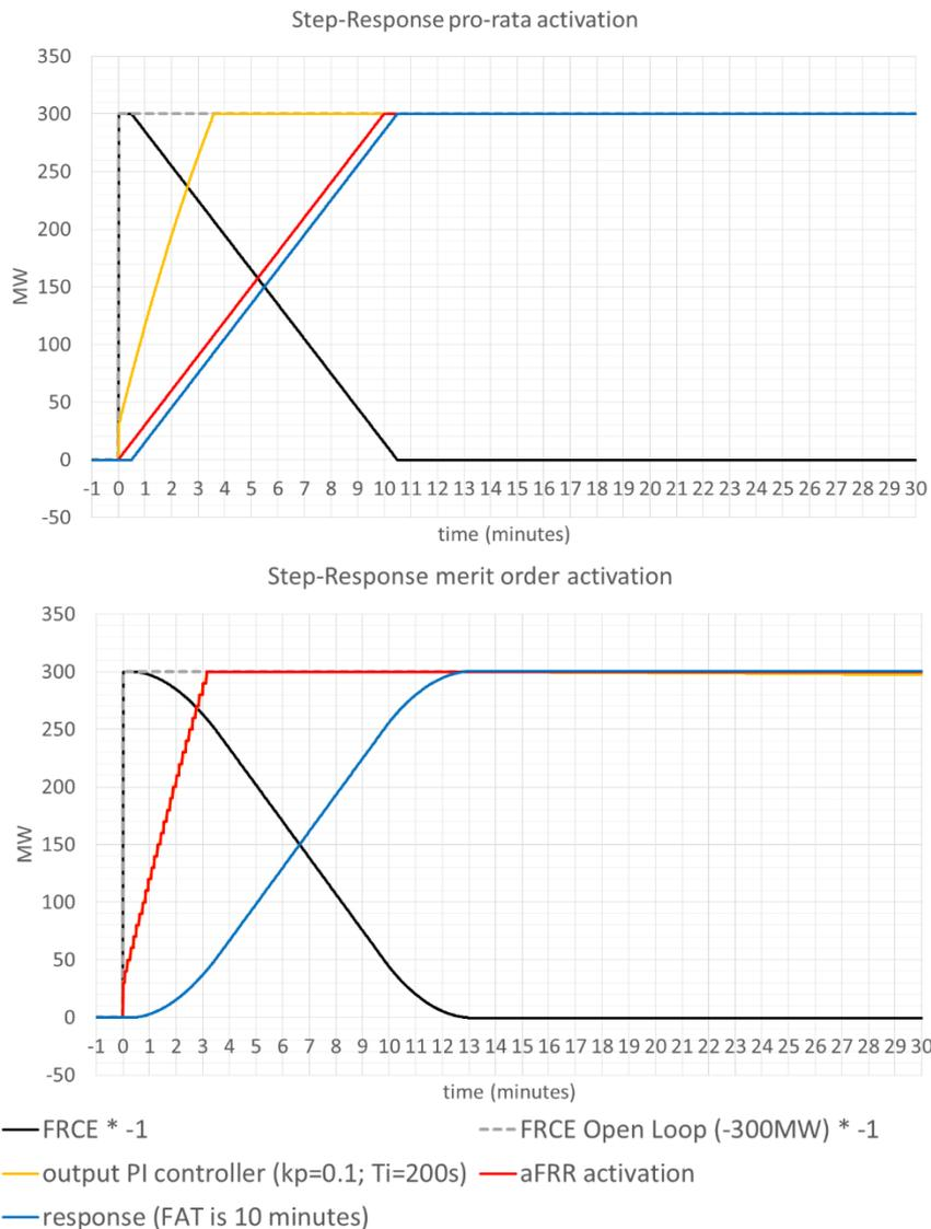
Figure 12: Large deviation (300MW step response) for pro-rata (upper figure) and merit-order (lower figure) activation scheme (300MW of aFRR connected to the LF Controller) <sup>12, 17</sup>.
