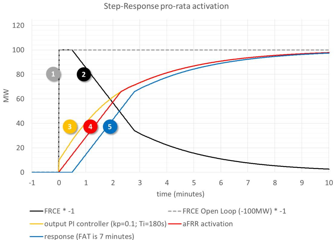
Figure 4: Typical response of generic automatic frequency restoration process to a 100MW generation trip<sup>12</sup>
