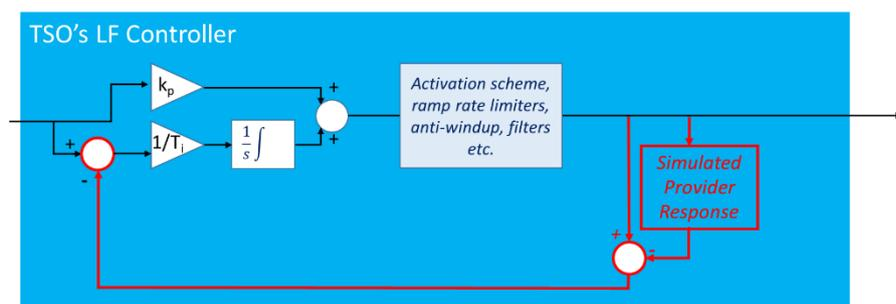
Figure 17: Simplified scheme that feeds back the expected response of aFRR providers
