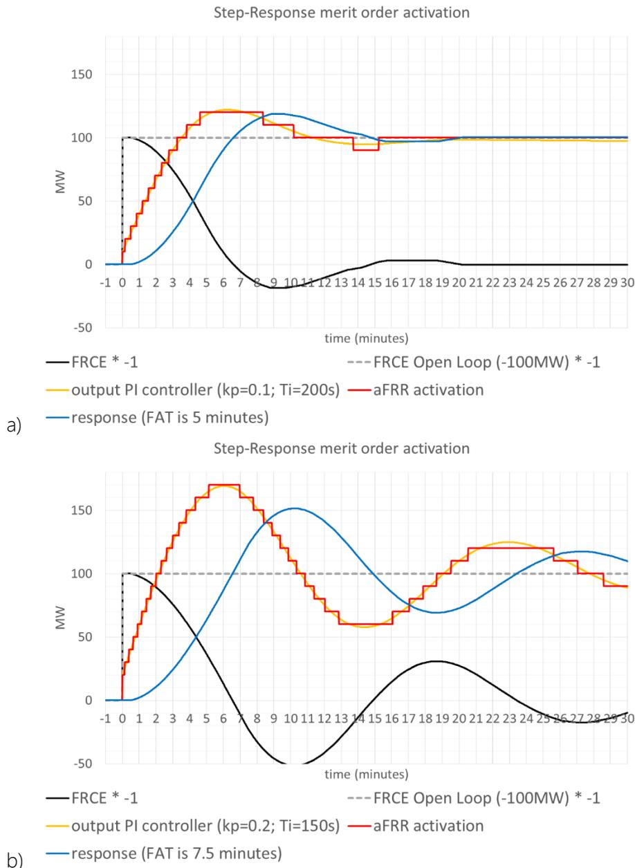
Figure 16: Step response for 100MW step of merit-order activation scheme with a smaller FAT: FAT is reduced from 10 minutes to 5 minutes in figure a) and to 7.5 minutes in figure b) (to be compared with Figure 11) <sup>12, 17</sup>.
