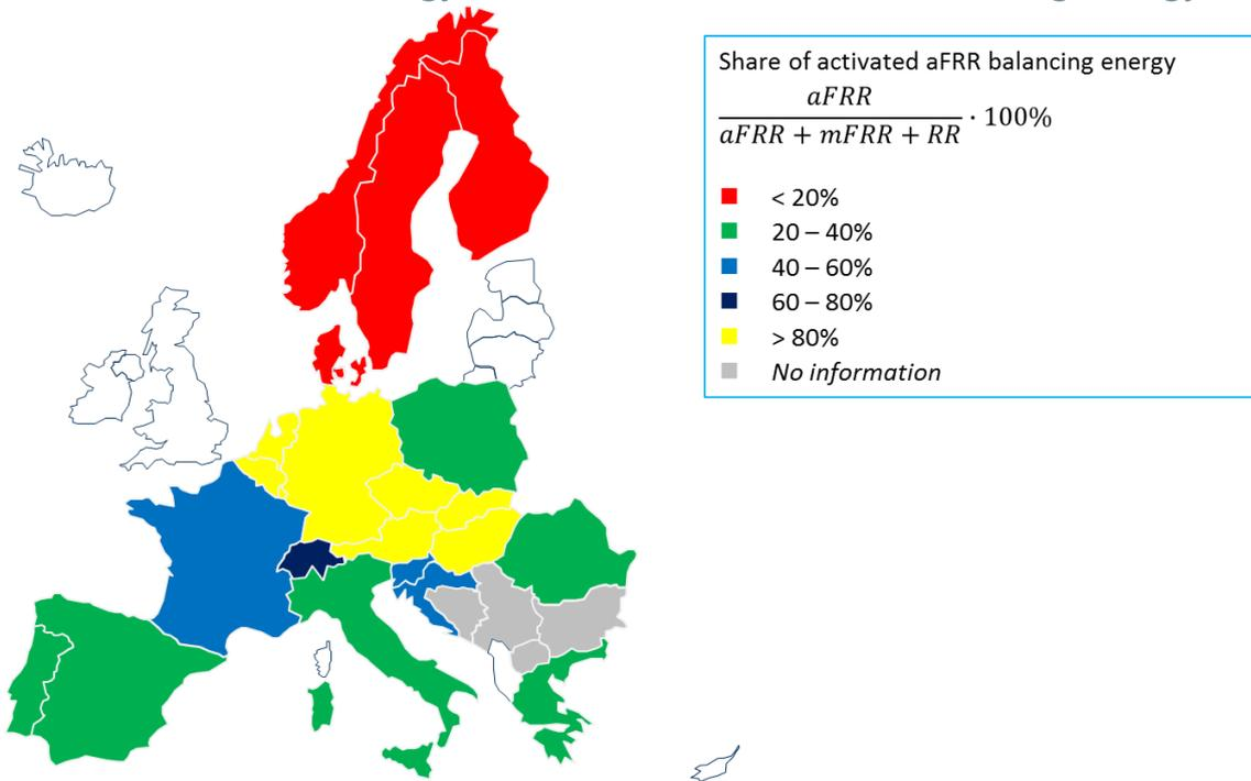
Figure 2: Share of aFRR energy in total activated FRR/RR balancing energy, based on figures for February and June 2015<sup>9</sup>.
