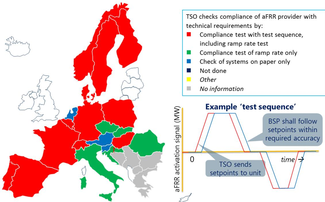
Figure 35: Compliance check: Prequalification tests
