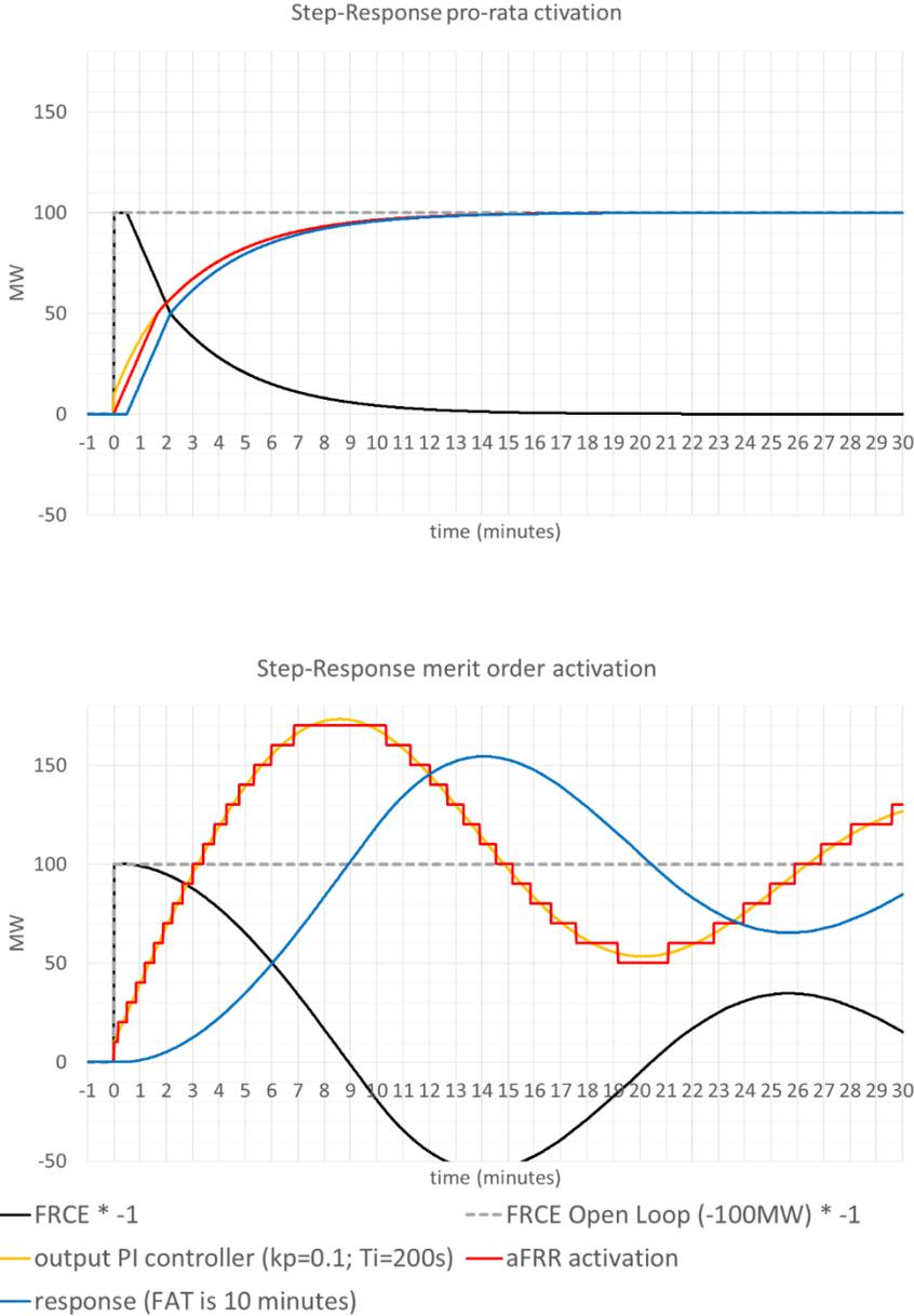
Figure 11: Small deviation (100MW step response) for pro-rata (upper figure) and merit-order (lower figure) activation scheme (300MW of aFRR connected to the LFC) <sup>12, 17</sup>.
