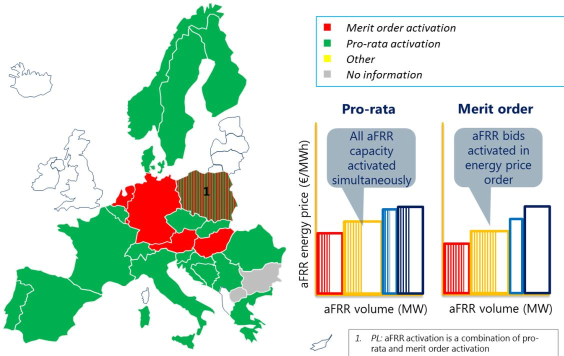
Figure 32: TSOs that apply a pro-rata activation scheme or a merit-order activation scheme
