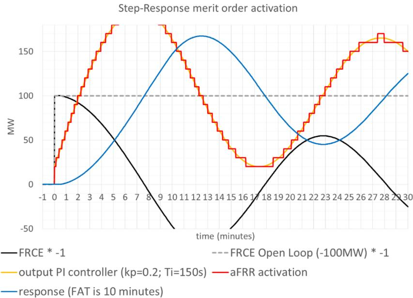
Figure 19: Step response for 100MW step of merit-order activation scheme with a smaller integration time  $T_i$  (to be compared with Figure 11) <sup>12, 17</sup>
