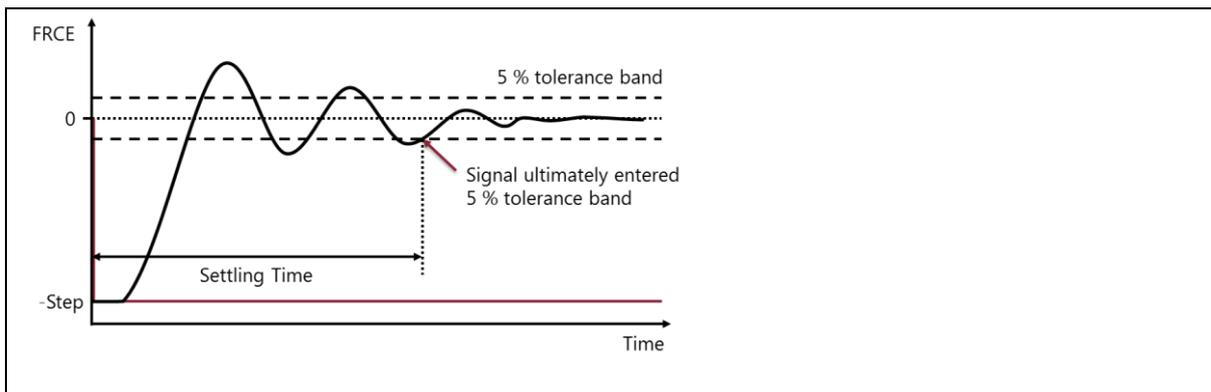
Figure 14: Calculation of settling time
