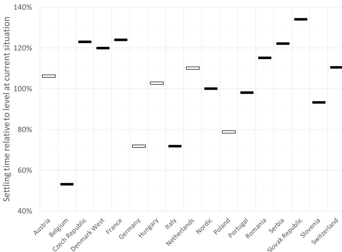
Figure 15: Settling time for large deviations for a simple merit order, relative to the settling time for the existing situation (open boxes show LFC Blocks that currently apply other merit order activation schemes)<sup>24</sup>
