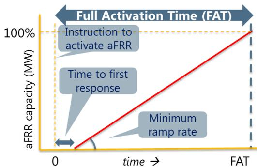
Figure 8: Conversion of time to first response and a minimum ramp rate to aFRR Full Activation Time
