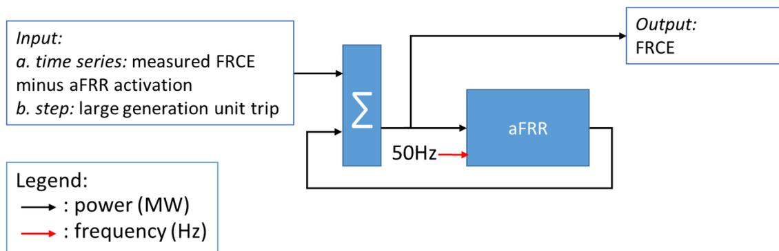
Figure 37: High level Matlab/Simulink model of the individual LFC Blocks in the CE system
