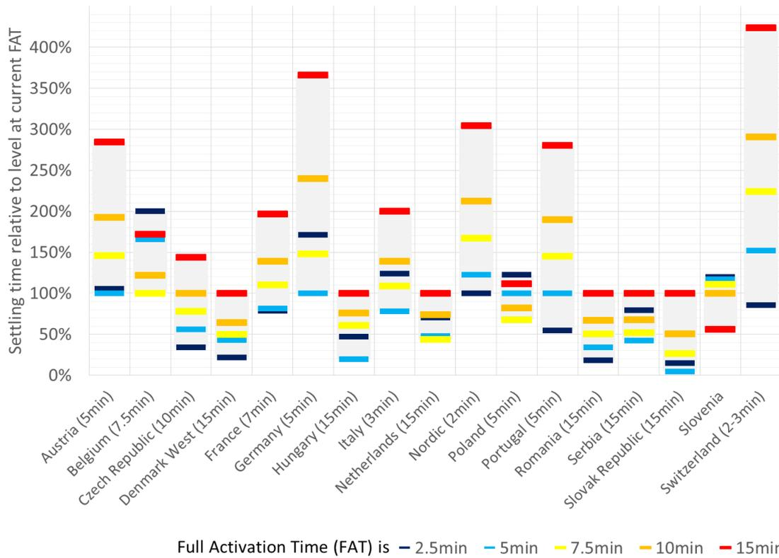
Figure 23: Settling time for a change from the existing FAT to a FAT of 2.5, 5, 7.5, 10 and 15 minutes, relative to the situation with a simple merit order activation scheme and the existing FAT (between brackets, the existing FAT) <sup>22</sup>
