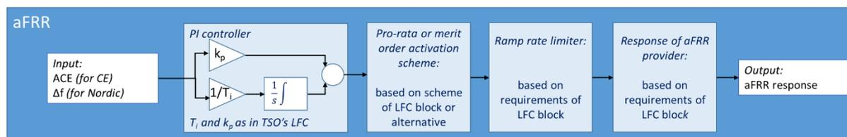
Figure 38: Simplified version of Matlab/Simulink aFRR model
