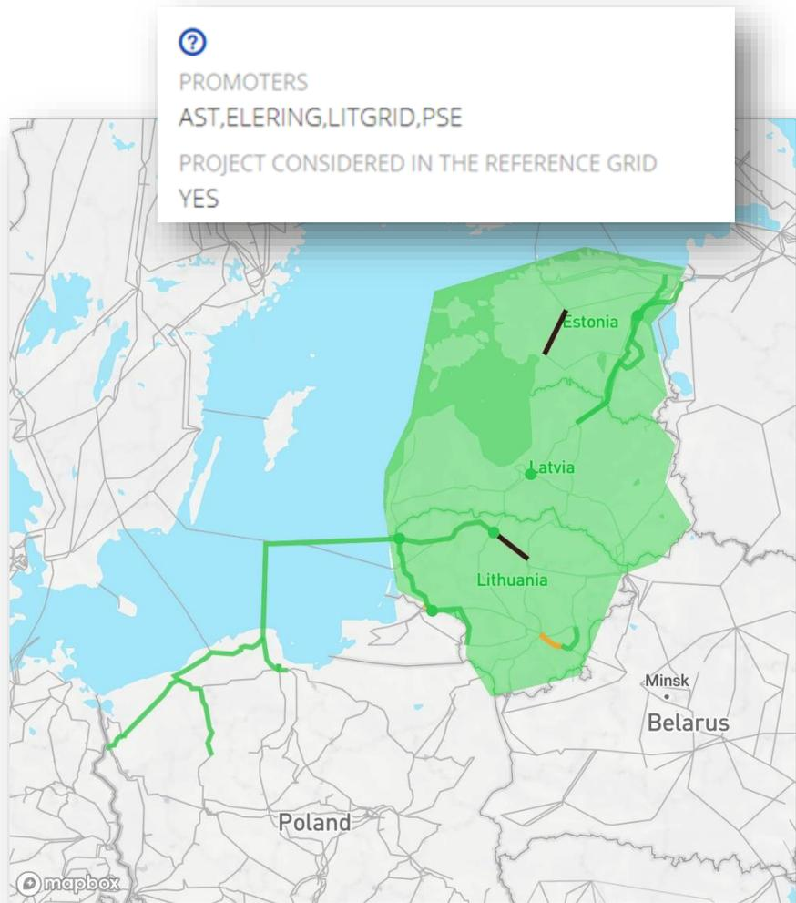
The three Baltic TSOs are preparing for desynchronization from IPS/UPS by 2025 and synchronization with the Continental European Network (CEN) through current DC interconnection between Lithuania and Poland.
