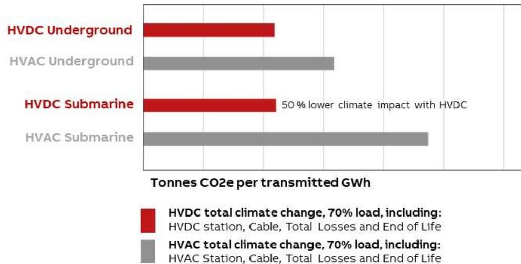
\*100 km submarine cable 900MW, German electricity mix
