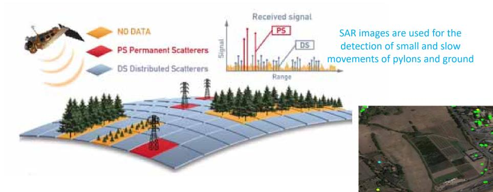
Displacement map using satellite SAR data
