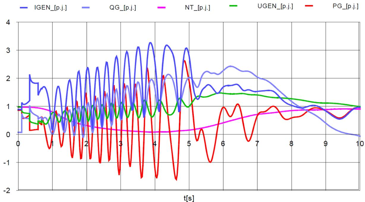
**FIGURE 8-11: SIMULATION OF HYPOTHETIC LOSS OF STABILITY**
