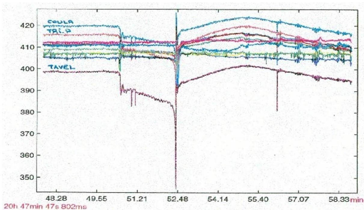
**Figure 8-14 : Voltage at several busses during the transient after fault**
