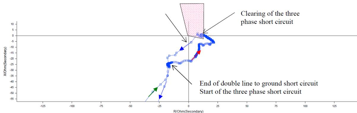
**FIGURE 8-9: TRAJECTORY OF APPARENT IMPEDANCE MEASURED IN THE SLAVĚTICE SUBSTATION**
