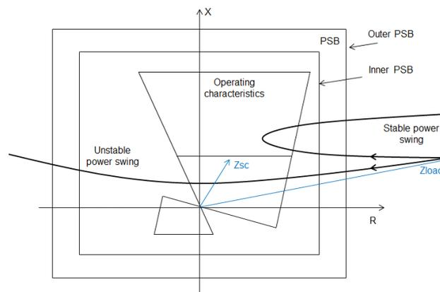
**Figure 6-1: Impedance diagram for impedance based PSB**
