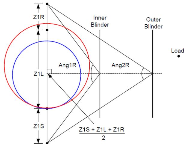
**Figure 6-2 Equivalent two-Source machine angles during unstable power swing**
