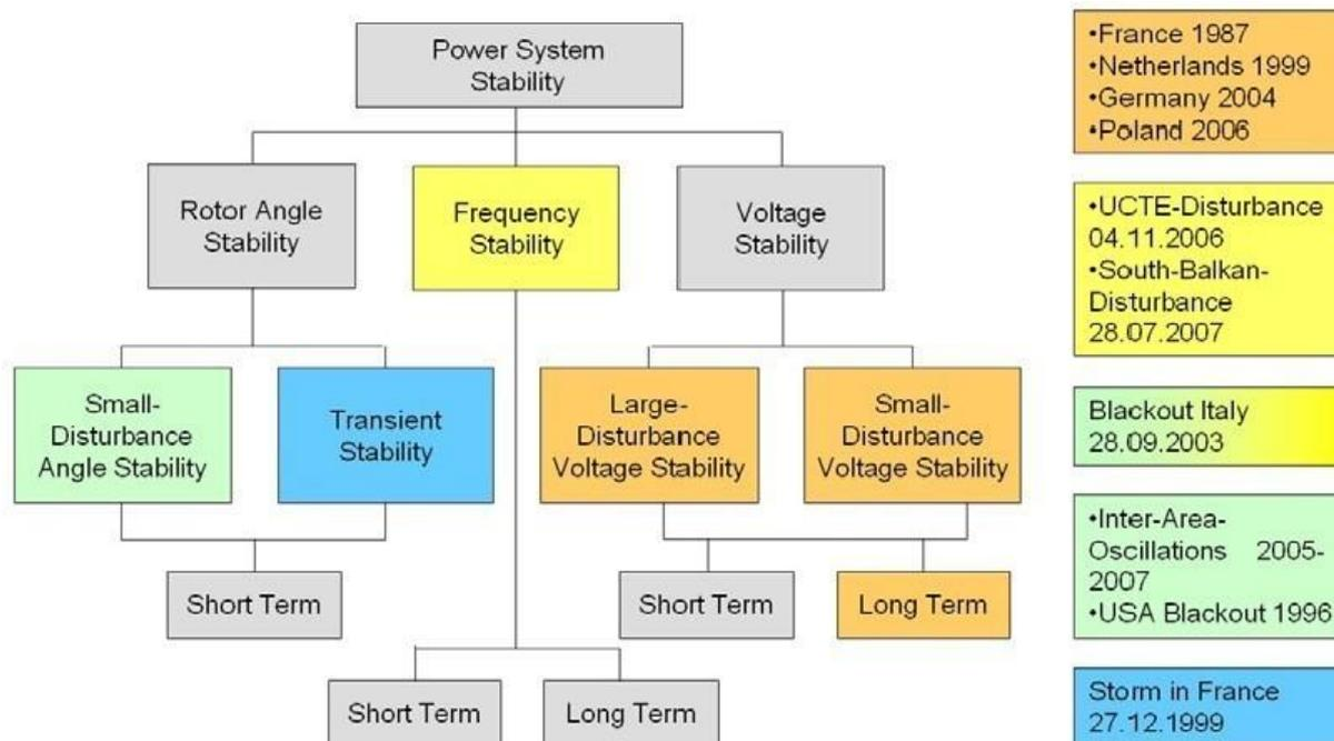
**Figure 2-2: Illustration of instability phenomena**
