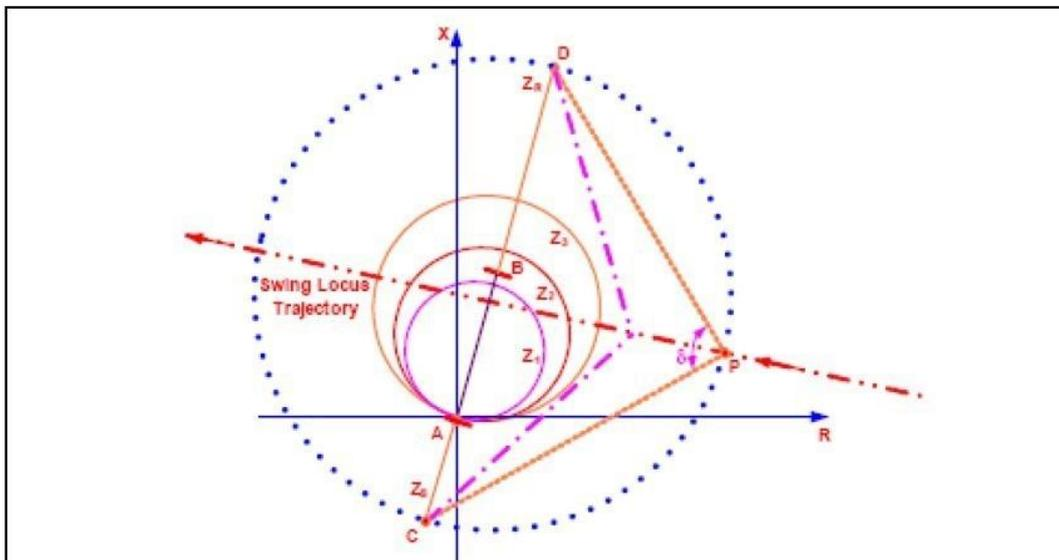
**Figure 3-2: Swing locus trajectory when the magnitude of ES/ER = 1.0**
