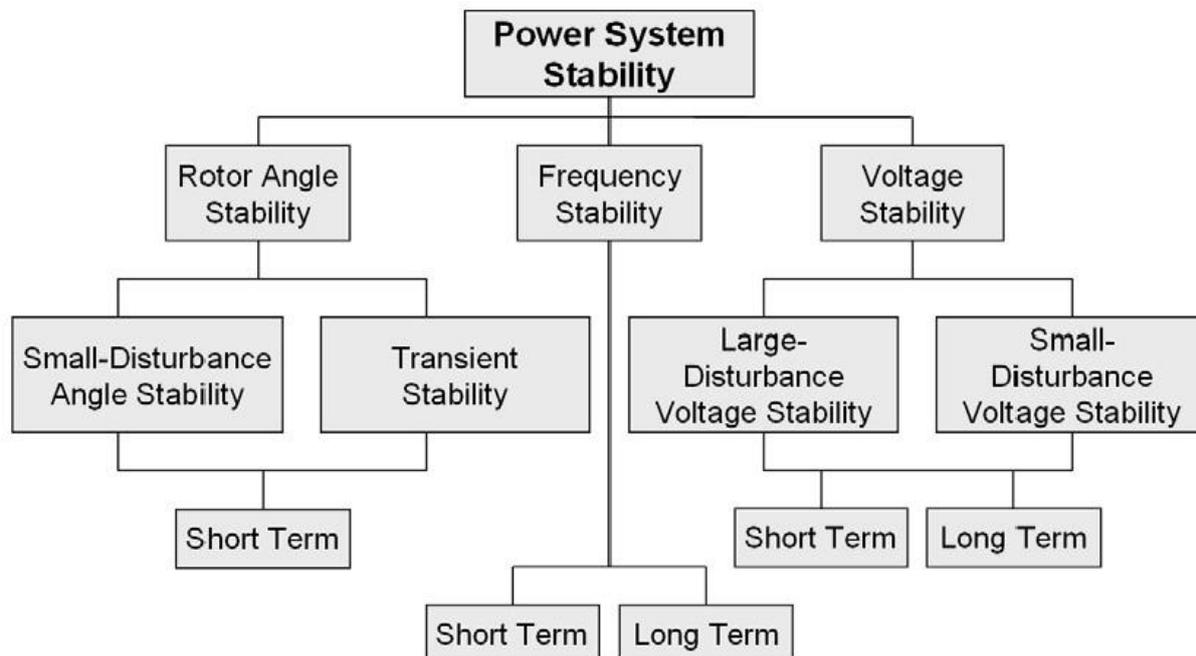
Figure 2-1: Classification of power system stability
