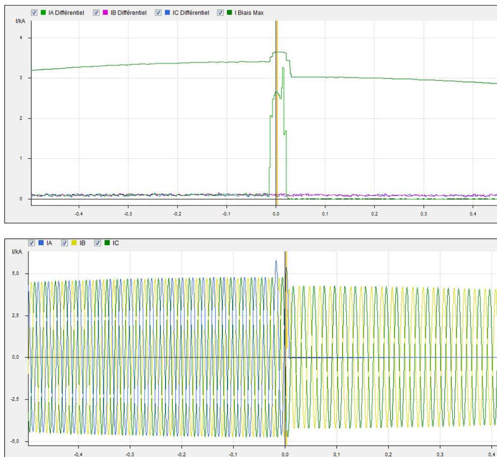
Figure 3-3: Restrain current (IBiais) and differential current (IA Différentiel) for a phase to ground fault on an 225 kV underground cable during an unstable power swing (0.2 Hz)
