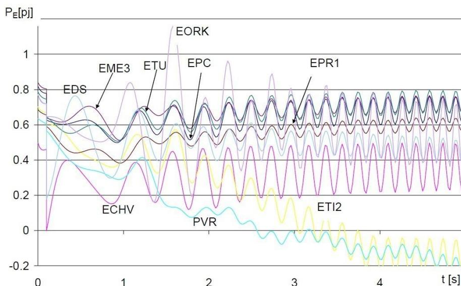
**FIGURE 8-7: CALCULATED OUTPUTS OF POWER STATIONS CONNECTED INTO AFFECTED PART OF NETWORK**
