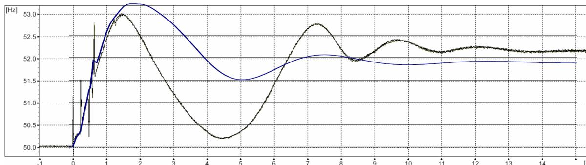
**FIGURE 8-10: MEASURED AND CALCULATED FREQUENCY TIME COURSE DURING PASSING INTO ISLAND**
