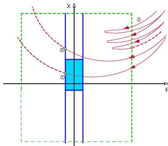
**Figure 7-1 Out-of-Step protection**
