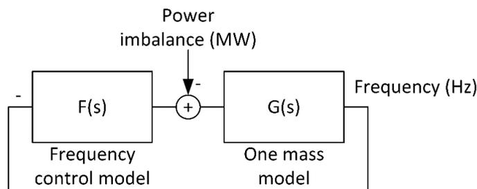
Figure 8 : Simple illustration of one mass model
