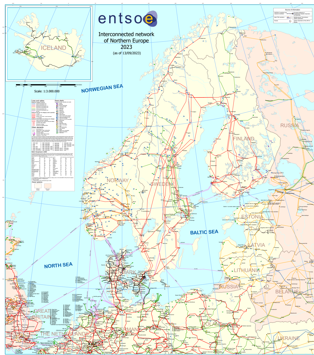
Figure 1.1: The Nordic and Baltic main grids [3] in 2023. All of Denmark is included in the disturbance data of this report although only the grid of eastern Denmark belongs to the Nordic synchronous area.
