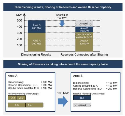
Suppose that the Dimensioning Rules for Area A and Area B result in the need of 300 MW FRR for Area A and 200 MW for Area B (same amounts as in Fejl! Henvisningskilde ikke fundet.). Without the sharing of reserve capacity, the TSOs of Area A and Area B have to ensure the availability of respectively 300 MW and 200 MW.
