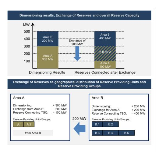
Suppose that the dimensioning results in the need of 300 MW for Area A and 200 MW for Area B. Without the exchange of reserve capacity, the respective reserve capacity has to be provided by reserve providing units or reserve providing groups connected to the Area which means that 300 MW have to be connected in Area A and 200 MW in Area B.
