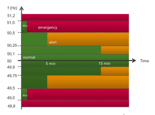
The figure above shows the definition of the different systems states with regard to system frequency in SOGL article 18 and Table 1 'Frequency quality defining parameters of the synchronous areas' in annex III of the SOGL. The figure is developed assuming an incident at time zero. This Annex and SOGL apply to the Normal and Alert State. The annex on Emergency and Restoration and the Network Code on Emergency and Restoration apply to the Emergency State.
