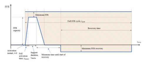
The figure illustrates the sequential diagram for the activation of FFR
