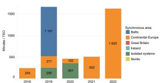
Figure 5.6: Operational security indicator OS-E1 from 2018–2022. It is calculated by adding up the duration of RRC0, RRC1 and RRC2 incidents and the duration of all other scale 0–3 incidents if a reduction of reserve capacity is reported, and dividing by the number of TSOs in the synchronous area.
