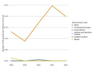
Figure 3.15: The annual number of OV-events per 100 km of installed circuit length in each synchronous area from 2018–2022.
