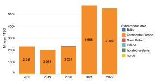
Figure 5.8: Operational security indicator OS-F1 from 2018–2022. It is calculated by adding up the duration of OVBS, OV0, OV1 and OV2 incidents and the duration of all other incidents on below scale and scale 0–3 where voltage deviations exceed the ranges from SOGL Annex II [1] are reported, and dividing by the number of TSOs in the synchronous area.
