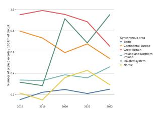
Figure 3.7: The annual number of scale 0 events per 100 km of circuit length from 2018–2022.
