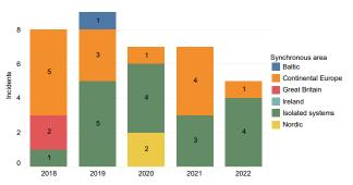
Figure 5.15: Operational security indicator OPS-C annually from 2018–2022. It is calculated by counting the number of scale 0-3 incidents where an exceptional contingency degraded the system operation state.
