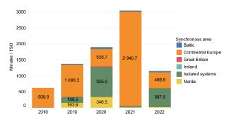
Figure 5.4: Operational security indicator OS-D1 from 2018–2022. It is calculated by adding up the number of minutes in alert and emergency states of all reported scale 0–3 incidents, and dividing by the number of TSOs in the synchronous area.
