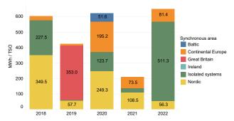
Figure 5.3: Operational security indicator OS-C from 2018–2022. It is calculated by adding up the reported energy not supplied due to unscheduled disconnection of demand facilities for all scale 0–3 incidents, and dividing by the number of TSOs in the synchronous area.
