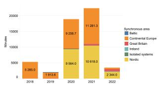
Figure 5.10: Operational security indicator OS-G1 from 2018–2022. It is calculated by adding up the number of minutes outside the standard frequency range for all scale 0–3 incidents.
