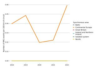
Figure 3.16: The annual number of RRC-events per 100 km of installed circuit length in each synchronous area from 2018–2022.
