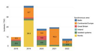
Figure 5.5: Operational security indicator OS-D2 from 2018–2022. It is calculated by counting the number of scale 0–3 incidents in which an alert or emergency state was reported, and dividing by the number of TSOs in the synchronous area.
