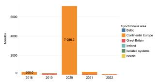
Figure 5.11: Operational security indicator OS-G2 from 2018–2022. It is calculated by adding up the number of minutes outside the 50% of maximum steady-state frequency deviation for all scale 0–3 incidents.
