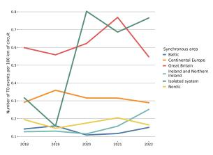
Figure 3.12: The annual number of T0-events per 100 km installed circuit length in each synchronous area from 2018–2022.
