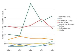
Figure 3.11: The annual number of T-events per 100 km installed circuit length in each synchronous area from 2018–2022.
