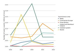
Figure 3.9: The annual number of scale 1 events per 100 km of circuit length from 2018–2022.
