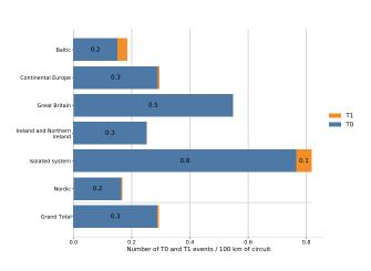
Figure 3.3: Number of events on transmission network elements (T0 and T1) per 100 km of circuit length in 2022.
