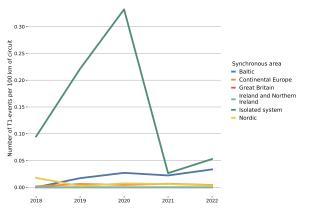
Figure 3.13: The annual number of T1-events per 100 km installed circuit length in each synchronous area from 2018–2022.
