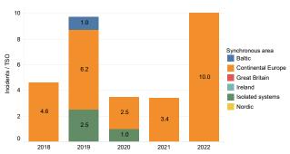
Figure 5.7: Operational security indicator OS-E2 from 2018–2022. It is calculated by counting the number RRC0, RRC1 and RRC2 incidents and the number of all other scale 0–3 incidents if a reduction of reserve capacity is reported, and dividing by the number of TSOs in the synchronous area.
