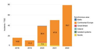
Figure 5.9: Operational security indicator OS-F2 from 2018–2022. It is calculated by counting the number of violation of standards of voltage incidents (OVBS, OV0, OV1 and OV2) and the number of all other below scale and scale 0–3 incidents in which the voltage standards are violated, and dividing by the number of TSOs in the synchronous area.
