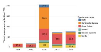
Figure 5.2: Operational security indicator OS-B from 2018–2022. It is calculated by adding up the number of tripped power generation facilities reported for scale 0-3 and below scale incidents and dividing by the number of TSOs in the synchronous area.
