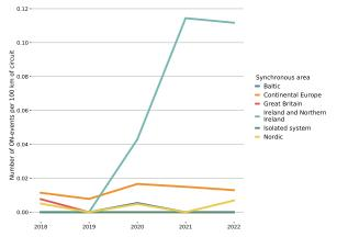
Figure 3.18: The annual number of ON-events per 100 km of installed circuit length in each synchronous area from 2018–2022.
