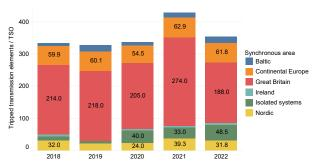
Figure 5.1: Operational security indicator OS-A from 2018–2022. It is calculated by adding up the number of tripped transmission system elements reported for all scale 0–3 incidents, and dividing by the number of TSOs in the synchronous area.
