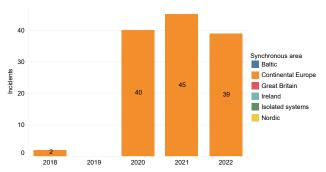
Figure 5.14: Operational security indicator OPS-B annually from 2018–2022. It is calculated by counting the number of OPS-A indicators where the cause was unexpected discrepancies from load and generation forecasts.
