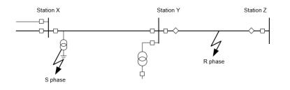
Figure 0.18 Double earth fault in a compensated network.
