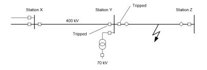
Figure 0.16 Line fault with unselective relay trip.
