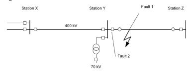
Figure 0.13 Line fault with simultaneous faults in surge arresters and circuit breaker.
