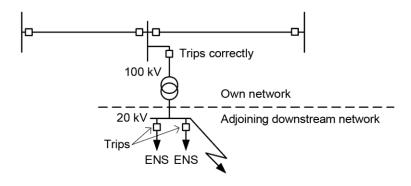
Figure 0.23 Fault on the lower side of a 100/20 kV transformer
