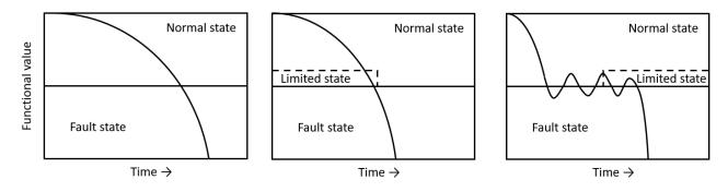
Figure 4.2 Transitioning from normal state or limited state to faults state is normally called a fault. If transition between states is intermittent, it is an intermittent fault.
