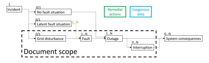
Figure 5.1 The situation after an incident is called a 'no fault situation', a 'latent fault situation' or a grid disturbance based on the involvement of faults. A grid disturbance is caused by faults and a fault can result in several outages. Outages can also result in none, one or several interruptions which may affect end-users and result in energy not supplied (ENS).
