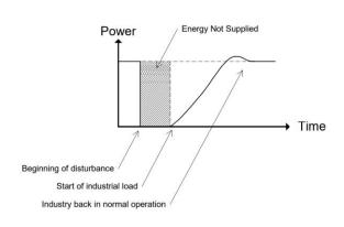
Figure 4.4 Grid disturbance with end-user interruption for industrial load. The interruption ends when voltage is supplied at the delivery point.
