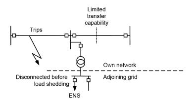
Figure 4.6 ENS due to transmission restrictions. A delivery point is disconnected because there is not enough transmission capacity.
