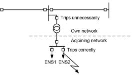
Figure 4.8 This scenario includes a breaker on the lower side of the transformer, in this case a breaker within the statistics trips unnecessarily. The ENS values should be separated If possible. The first ENS (ENS2) is for the line where the feeder tripped correctly (fault in another statistical area) and the other ENS (ENS1) is for the feeder where the breaker tripped unnecessarily.
