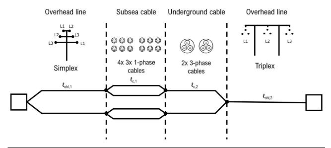
Figure 7.3 Circuit length and physical length calculation example of an HVAC overhead line and subsea/underground cable section. The diagram is a 3-phase single line. Circuit length only considers a single conductor length, ignoring parallel lines and cables, between the circuit breakers. Physical length for the overhead line sections multiplies the circuit length by the number of 3phase sets, and physical length for the cable sections multiply circuit length by the number of physical cables.
