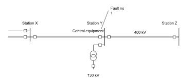
Figure 0.11 Unsuccessful power transformer energisation due to sensitive relay settings.
