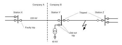
Figure 0.17 A fault in one company's network causing outage in another company's network.
