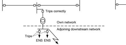
Figure 4.7 A failure in the downstream network causes an outage in a system unit within the statistical area resulting in ENS. As an outage causing ENS also occurs within the statistical area, this ENS must be included in the statistics with the fault sub-subcause 'Adjoining grid below 100 kV'.
