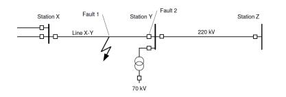
Figure 0.4 Line fault with a circuit breaker malfunction
