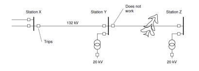
Figure 0.15 Fault on a radial feeder line with circuit breaker failing to trip.
