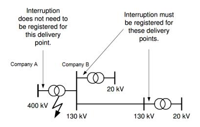
Figure 4.3 It is only the delivery points from the transmission network to low voltages that are registered
