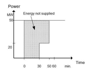
Figure 0.21 A visual representation of how to calculate the energy not supplied in the example of Section 0.
