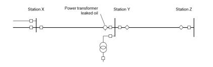
Figure 0.6 Manual line disconnection due to a faulty current transformer.
