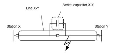
Figure 0.22 Outage of line with series capacitor.
