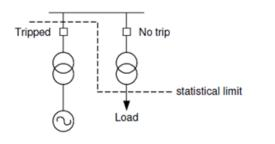
Figure 0.9 Fault in a generator connected directly to the transmission network
