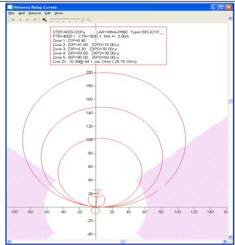
Figure 2: Load encroachment characteristic
