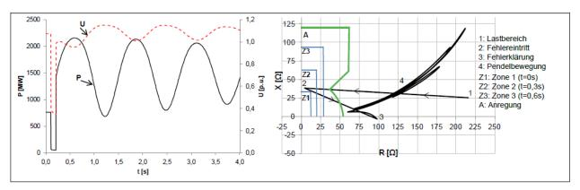
Figure 3. A Typical PSB characteristic in Z level (Source: "The Power Swing Blocking – a Solution for all oscillatory problems?" Martin Lösing, Klaus Vennemann, Rainer Krebs, VDE Conference, March 2011, Munich)
