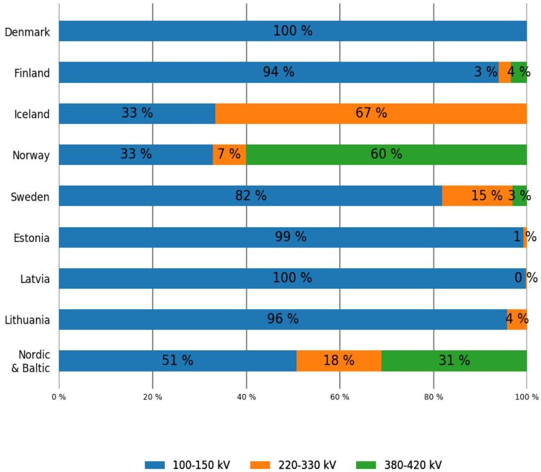
Figure 4.2.2 Percentage distribution of Energy not supplied in terms of the voltage level of the primary fault during the period 2007–2016 for the Nordic countries and Estonia and for the period 2012–2016 for Latvia and Lithuania
