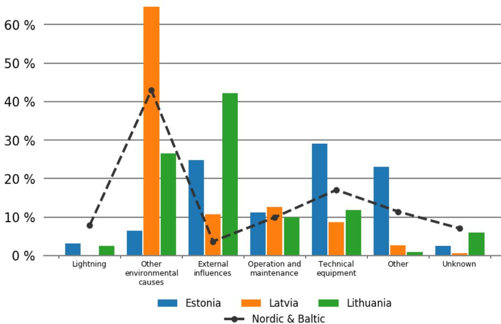
Figure 4.5.4 Average percentage distribution of ENS per the cause of the primary fault for Estonia during 2007–2016 and for Latvia and Lithuania during 2012–2016
