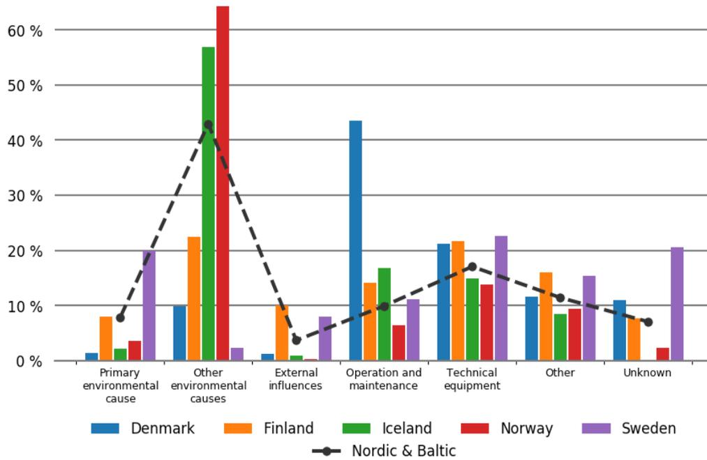
Figure 4.5.3 Average percentage distribution of ENS per the cause of the primary fault in each Nordic country during the period 2007–2016
