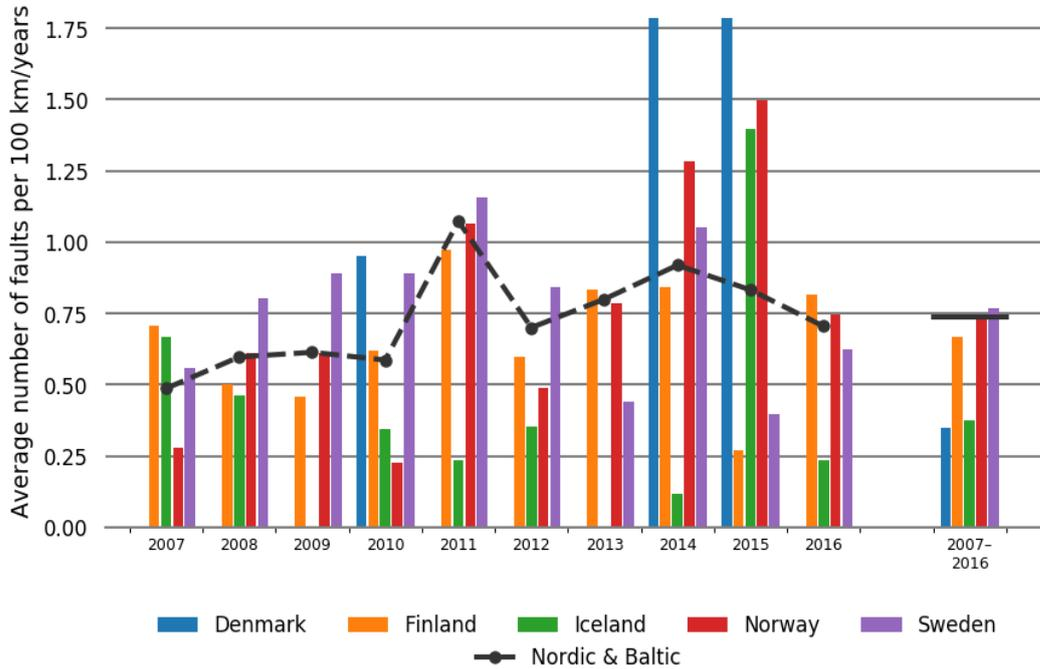
Figure 5.3.2 Annual distribution of faults for 220–330 kV overhead lines during the period 2007–2016 and the average for 2007–2016 in each Nordic country
