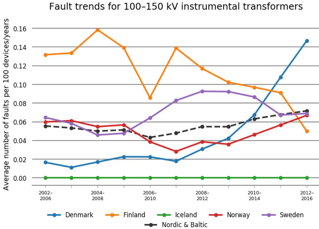
Figure 5.6.4 Fault trends as five-year averages for instrument transformers at the voltage level 100–150 kV in each Nordic country
