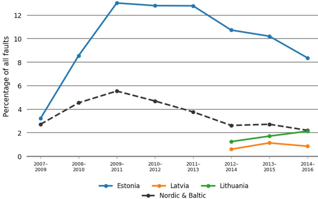
Figure 6.6.9 Fault trends as three-year averages for 100-150 kV operation and maintenance faults for each Baltic country. Estonia has reported data since 2007 and Latvia and Lithuania have reported data since 2012.
