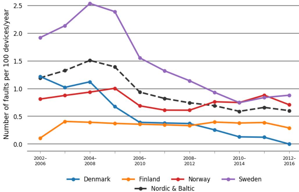
Figure 5.7.1 Fault trends as five-year averages for circuit breakers at the voltage level 380–420 kV in Nordic countries
