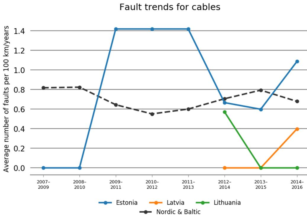
Figure 5.4.4 Fault trends as three-year averages for cables at all voltage levels in each Baltic country. Estonia has reported data since 2007 and Latvia and Lithuania have reported data since 2012.
