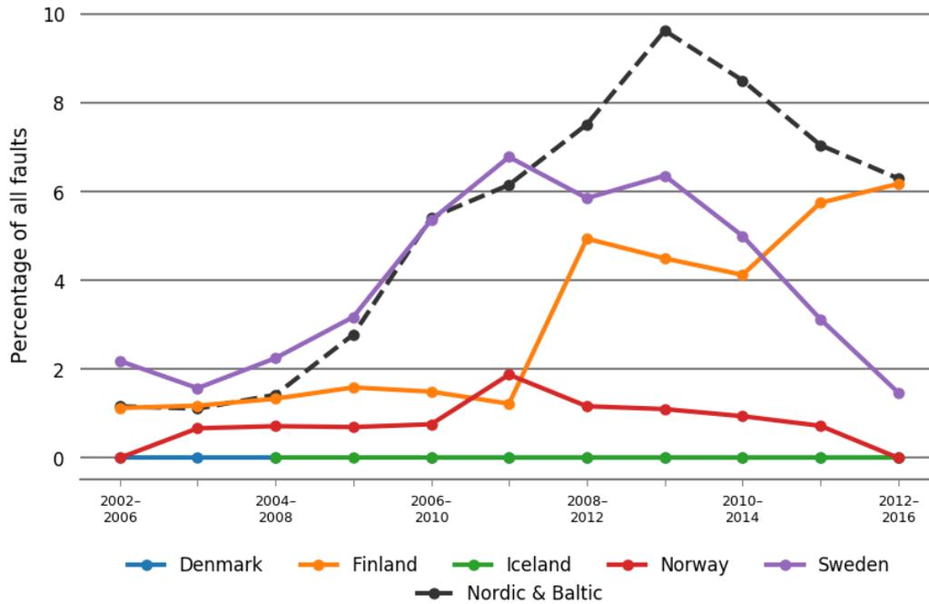
Figure 6.6.10 Fault trends as five-year averages for 220–330 kV operation and maintenance for each Nordic country
