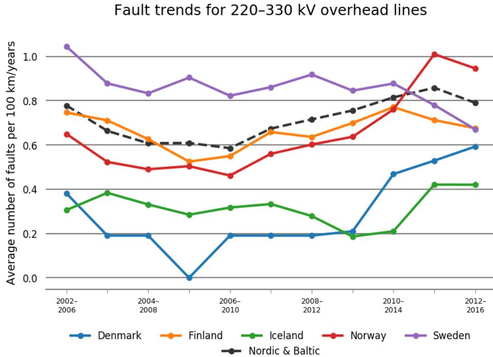
Figure 5.3.11 Fault trends as five-year averages for overhead lines at the voltage level 220–330 kV in each Nordic country
