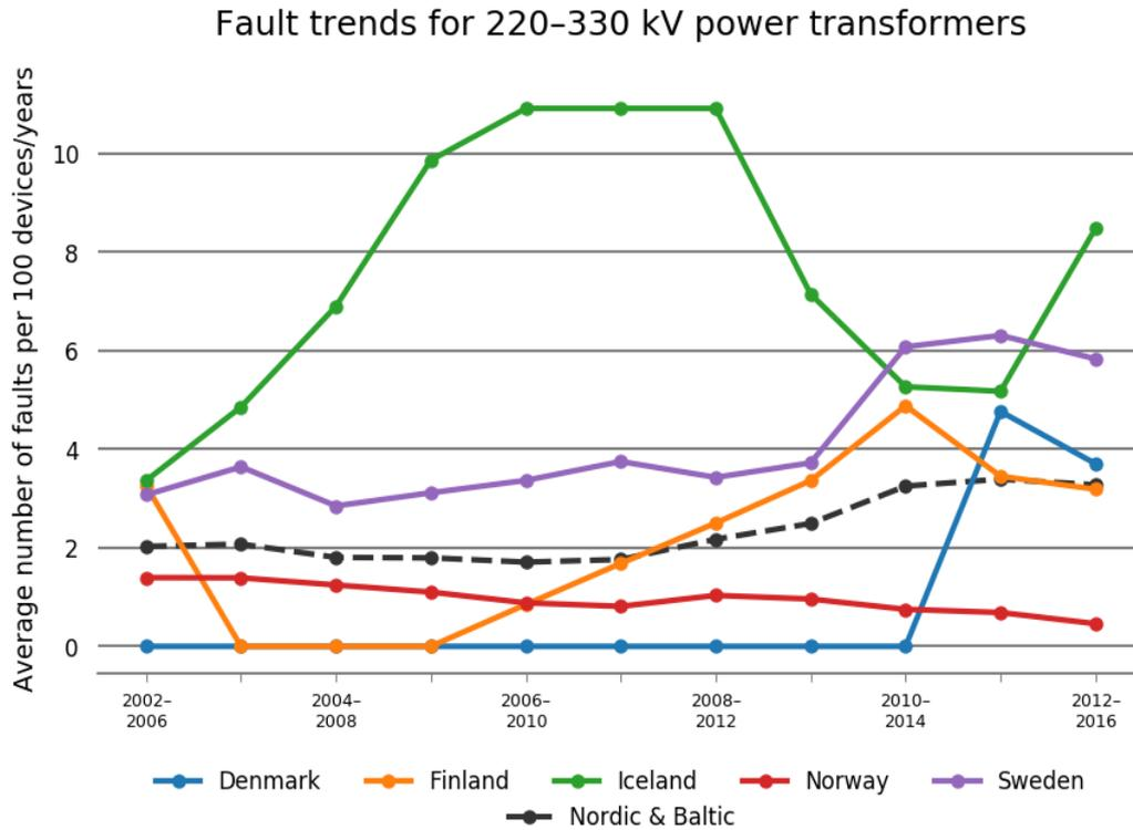
Figure 5.5.7 Fault trends as five-year averages for 220–330 kV power transformers in each Nordic country
