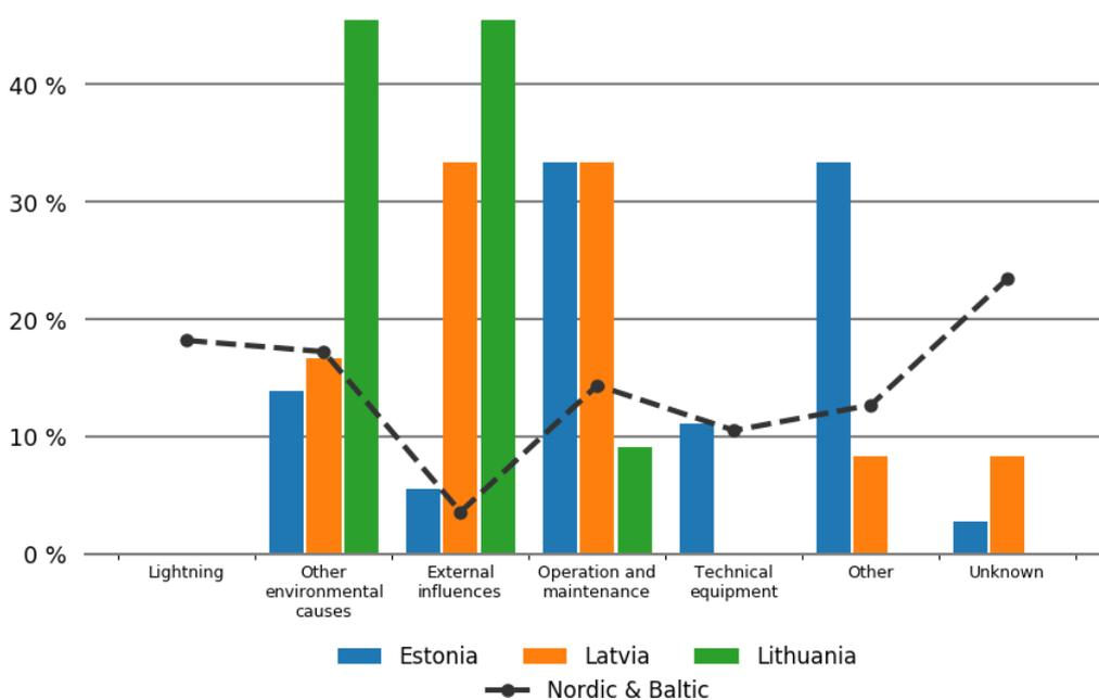
Figure 3.3.4 Percentage distribution of grid disturbances causing ENS per cause in each Baltic country in 2016
