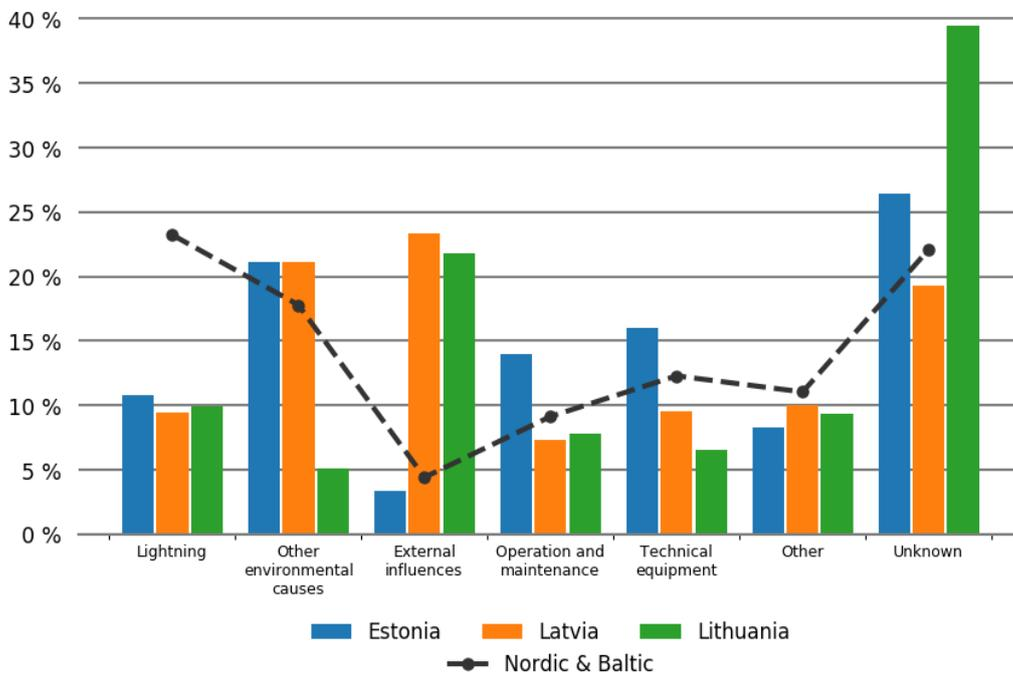
Figure 3.3.6 Average percentage distribution of grid disturbances per cause for Estonia during 2007–2016 and for Latvia and Lithuania during 2012–2016
