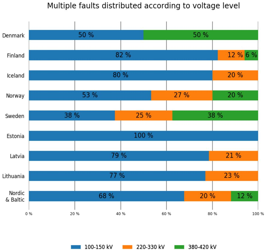
Figure 6.4.1 Percentage distribution of multiple fault situations in the Nordic and Baltic countries in 2016
