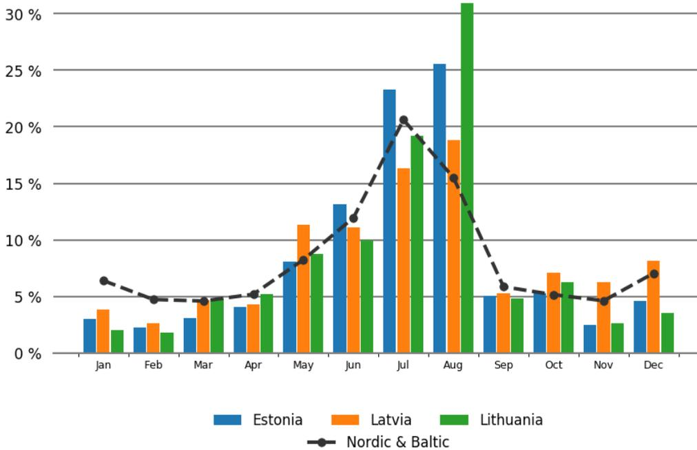
Figure 3.2.4 Average percentage distribution of grid disturbances per month for Estonia during 2007–2016 and for Latvia and Lithuania during 2012–2016
