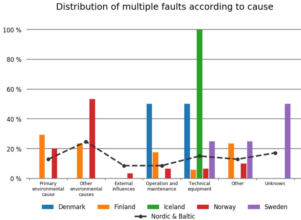
Figure 6.3.1 Percentage distribution of multiple fault situations per cause in the Nordic countries in 2016
