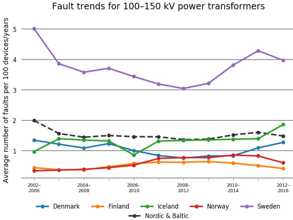
Figure 5.5.9 Fault trends as five-year averages for 100–150 kV power transformers in each Nordic country
