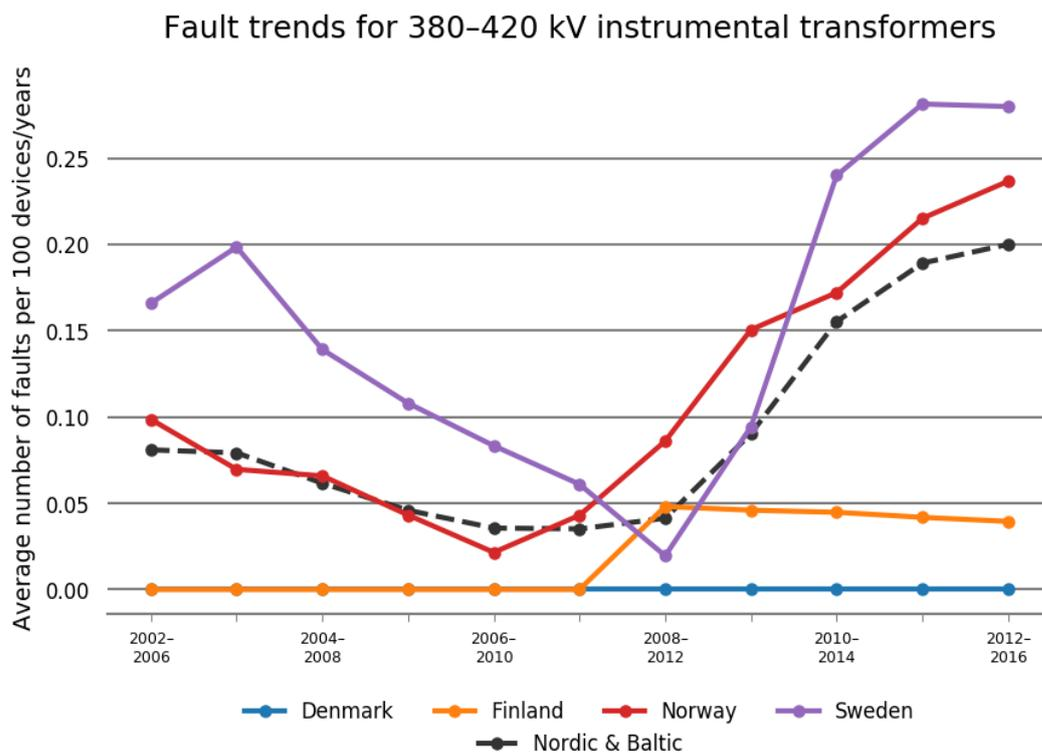
Figure 5.6.1 Fault trends as five-year averages for 380–420 kV instrument transformers in Nordic countries
