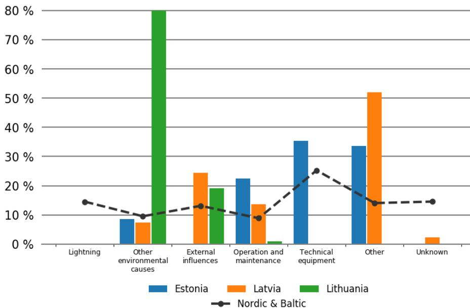
Figure 4.5.2 Percentage distribution of energy not supplied per the cause of the primary fault in each Baltic country in 2016
