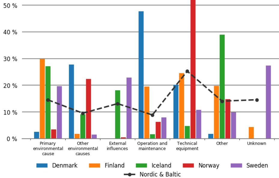
Figure 4.5.1 Percentage distribution of energy not supplied per the cause of the primary fault in each Nordic country in 2016
