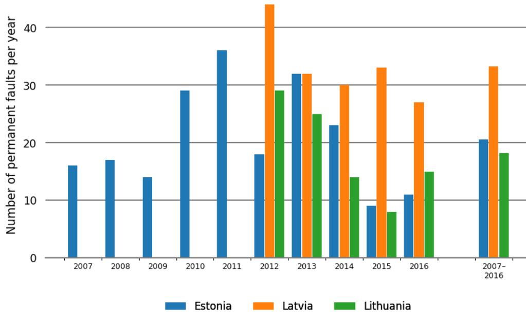
Figure 5.3.9 Annual distribution of permanent faults for 100–150 kV overhead lines during the period 2007–2016 and the average for Estonia during 2007–2016 and for Latvia and Lithuania during 2012–2016
