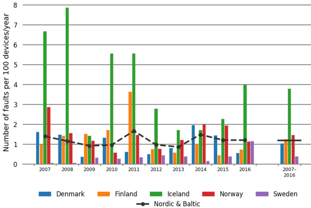
Figure 5.8.4 Annual distribution of 100–150 kV control equipment faults and the average for the period 2007–2016 for each Nordic country
