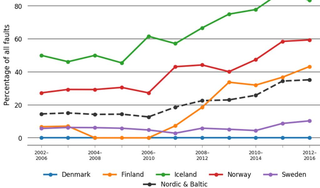
Figure 6.6.3 Fault trends as five-year averages for 220–330 kV other environmental causes for each Nordic country
