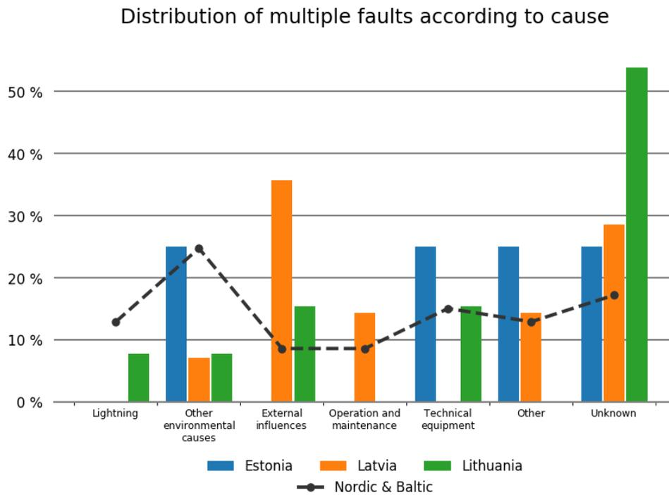
Figure 6.3.2 Percentage distribution of multiple fault situations per cause in the Baltic countries in 2016
