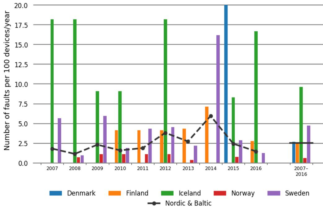
Figure 5.5.2 Annual distribution of faults for 220–330 kV power transformers in each Nordic country during the period 2007–2016
