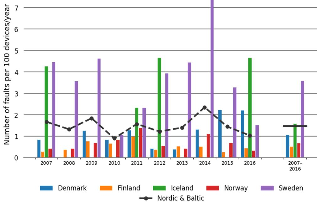
Figure 5.5.4 Annual distribution of faults for 100–150 kV power transformers in each Nordic country during the period 2007–2016
