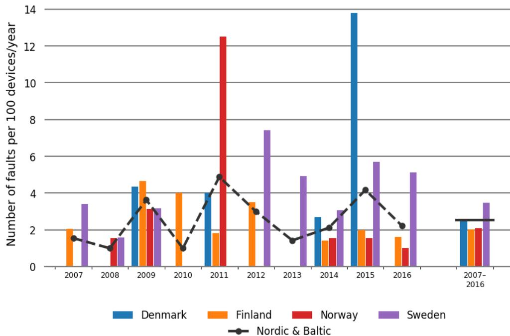
Figure 5.5.1 Annual distribution of faults for 380–420 kV power transformers in Nordic countries during the period 2007–2016
