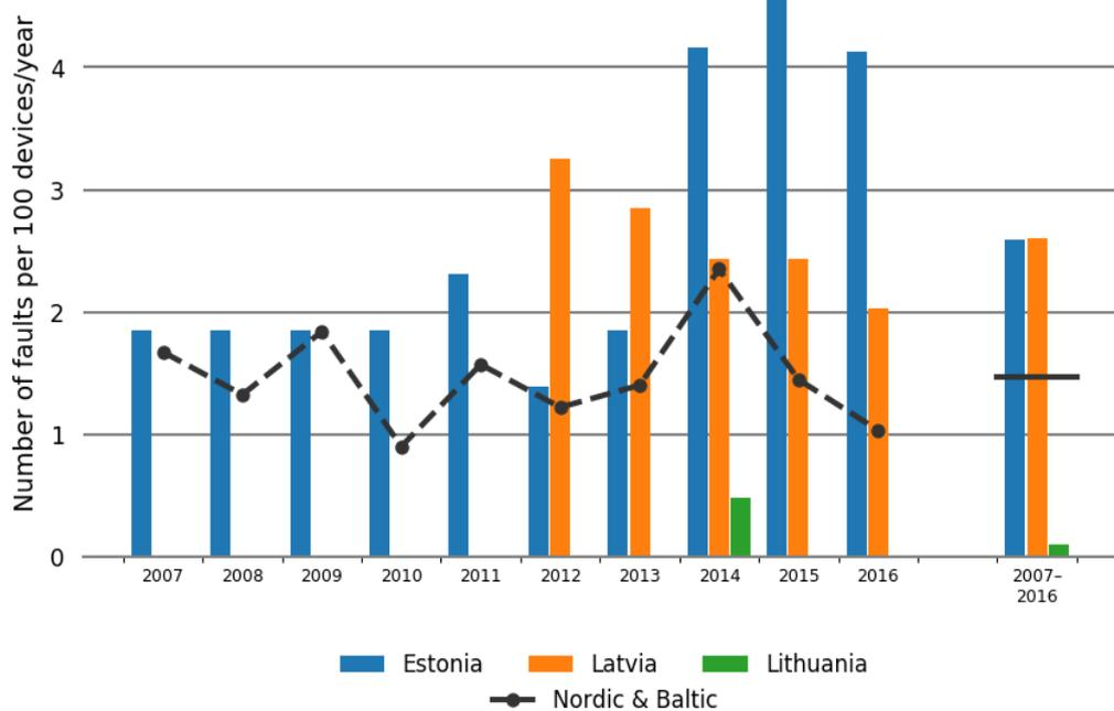
Figure 5.5.5 Annual distribution of faults for 100–150 kV power transformers and the average for Estonia during 2007–2016 and for Latvia and Lithuania during 2012–2016
