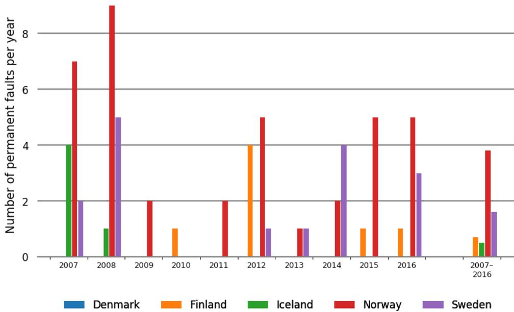
Figure 5.3.4 Annual distribution of permanent faults for 220–330 kV overhead lines during the period 2007–2016 and the average for 2007–2016 in each Nordic country
