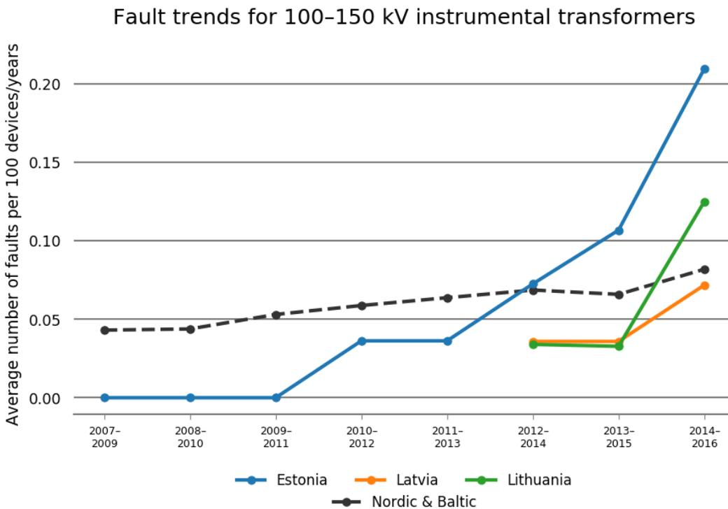
Figure 5.6.5 Fault trends as three-year averages for instrument transformers at the voltage level 100–150 kV in each Baltic country. Estonia has reported data since 2007 and Latvia and Lithuania have reported data since 2012.
