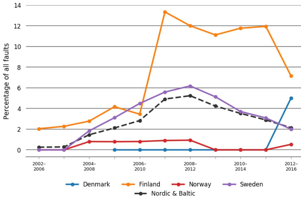
Figure 6.6.12 Fault trends as five-year averages for 380–420 kV operation and maintenance for each Nordic country
