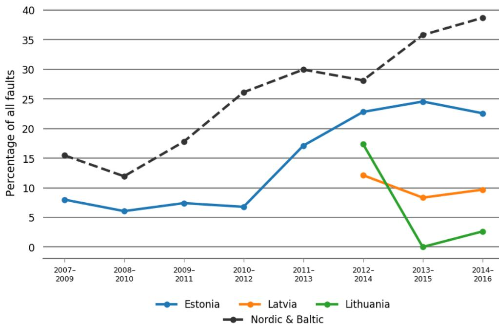
Figure 6.6.4 Fault trends as three-year averages for 220–330 kV other environmental causes for each Baltic country. Estonia has reported data since 2007 and Latvia and Lithuania have reported data since 2012.
