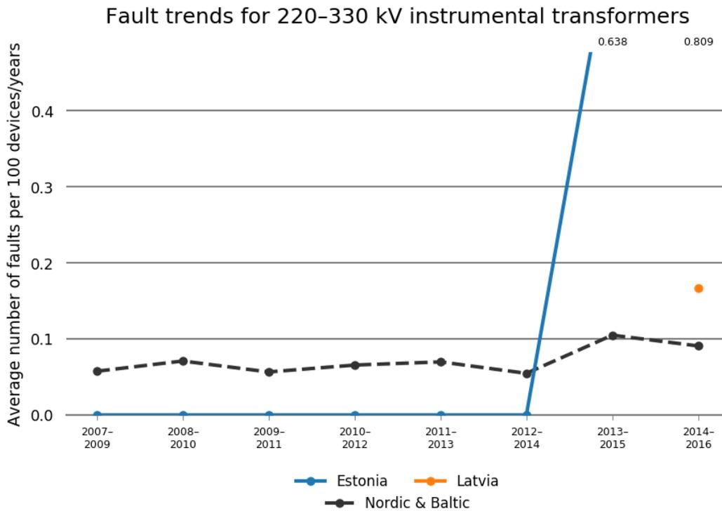
Figure 5.6.3 Fault trends as three-year averages for instrument transformers at the voltage level 220–330 kV in each Baltic country. Estonia has reported data since 2007 and Latvia and Lithuania have reported data since 2012.
