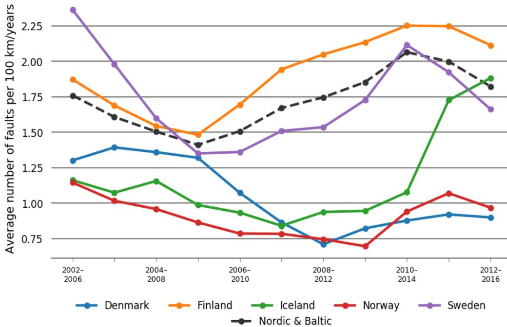
Figure 5.3.13 Fault trends as five-year averages for overhead lines at the voltage level 100–150 kV in each Nordic country
