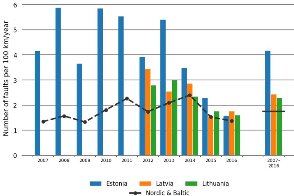
Figure 5.3.7 Annual distribution of line faults for 100–150 kV overhead lines during the period 2007–2016 and the average for Estonia during 2007–2016 and for Latvia and Lithuania during 2012–2016
