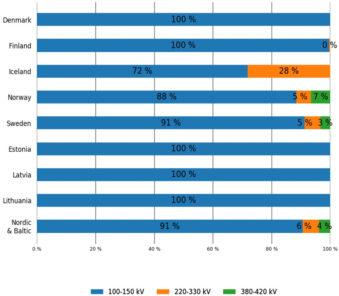
Figure 4.2.1 Percentage distribution of energy not supplied (ENS) in terms of the voltage level of the primary fault in 2016
