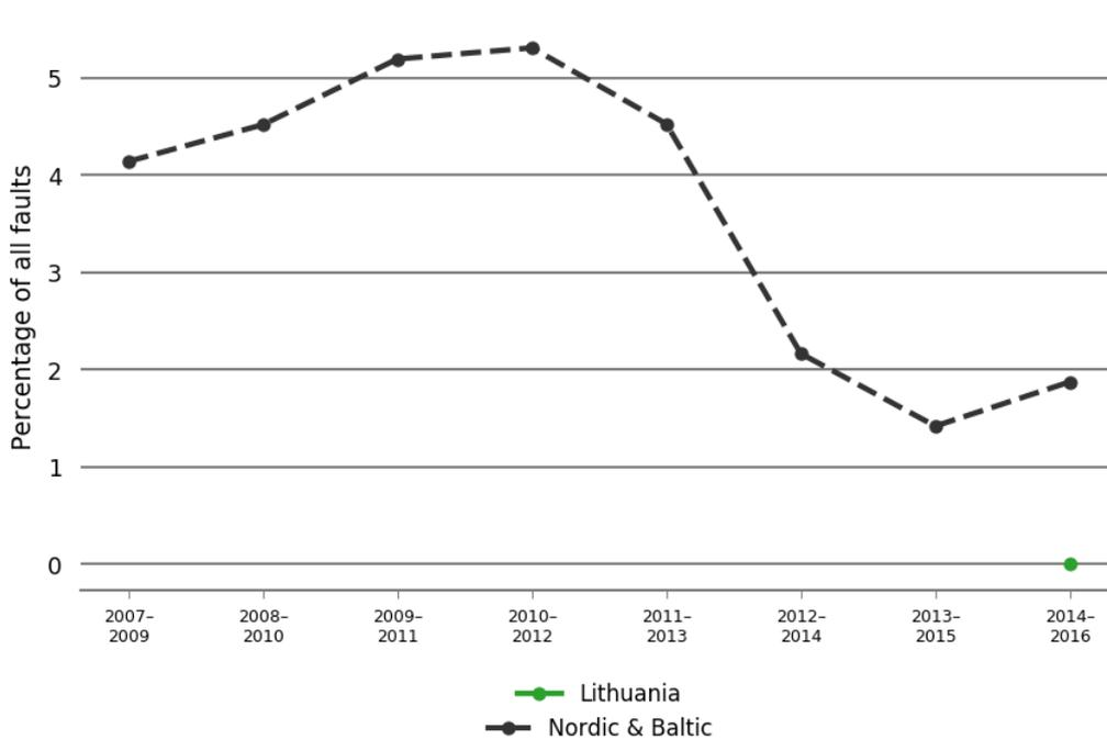
Figure 6.6.13 Fault trends as three-year averages for 380–420 kV operation and maintenance for Lithuania. Lithuania has reported data since 2012.
