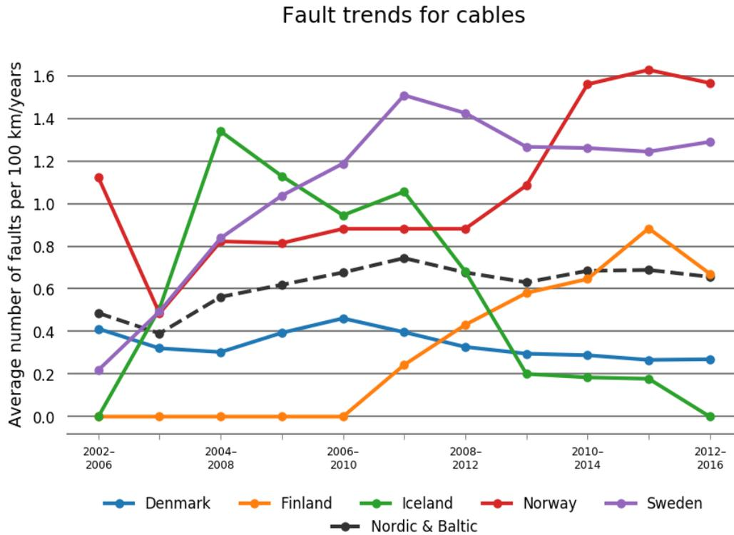
Figure 5.4.3 Fault trends as five-year averages for cables at all voltage levels in each Nordic country
