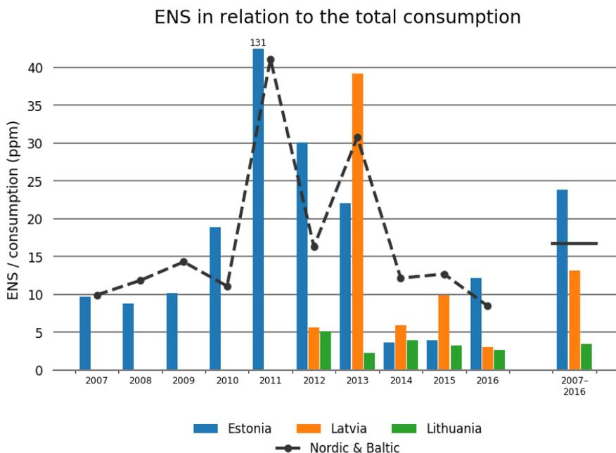
Figure 4.3.2 Annual energy not supplied (ENS) divided by consumption (ppm) for Estonia during 2007–2016 and for Latvia and Lithuania during 2012–2016
