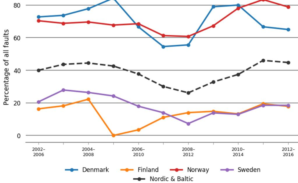
Figure 6.6.5 Fault trends as five-year averages for 380–420 kV other environmental causes for each Nordic country
