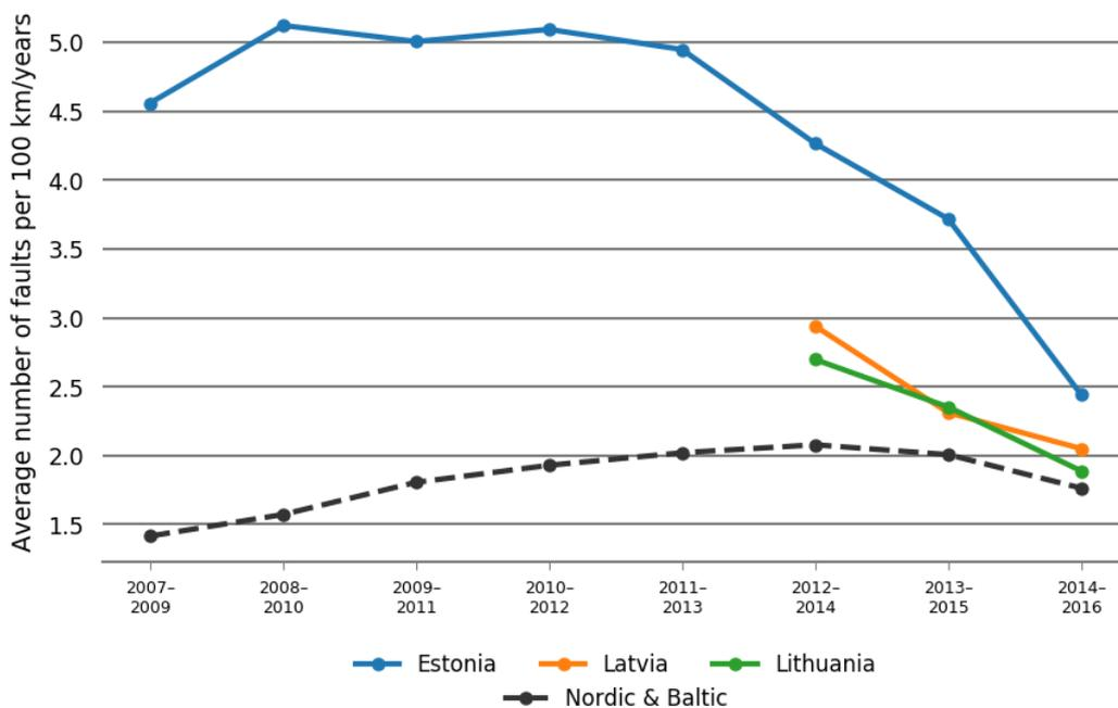
Figure 5.3.14 Fault trends as three-year averages for overhead lines at the voltage level 100–150 kV in each Baltic country. Estonia has reported data since 2007 and Latvia and Lithuania have reported data since 2012.
