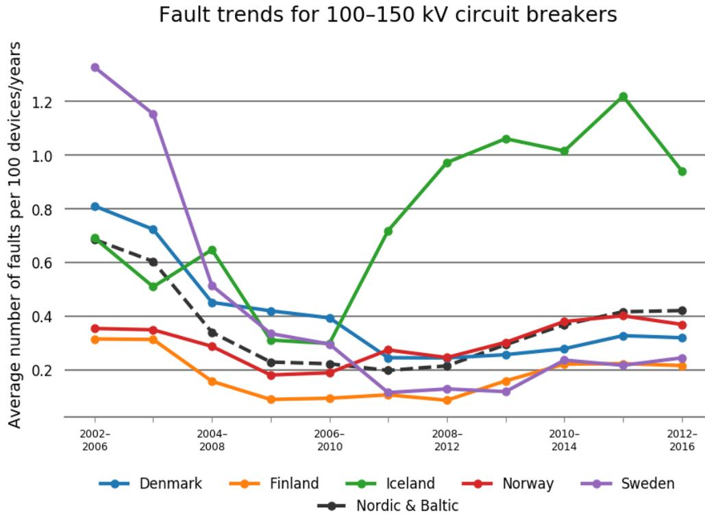
Figure 5.7.4 Fault trends as five-year averages for circuit breakers at the voltage level 100–150 kV in each Nordic country
