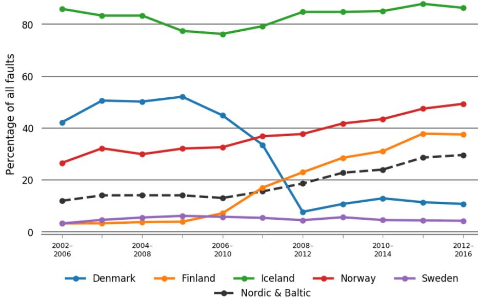
Figure 6.6.1 Fault trends as five-year averages for 100–150 kV other environmental causes for each Nordic country
