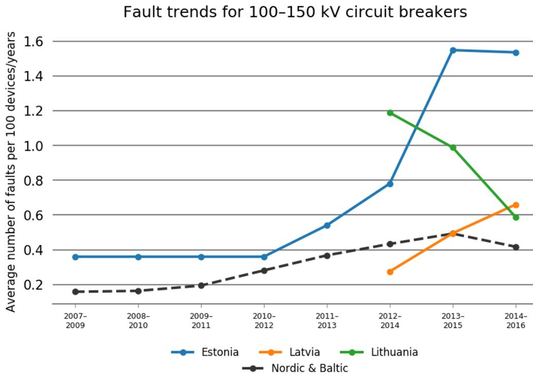
Figure 5.7.5 Fault trends as three-year averages for circuit breakers at the voltage level 100–150 kV in each Baltic country. Estonia has reported data since 2007 and Latvia and Lithuania have reported data since 2012.
