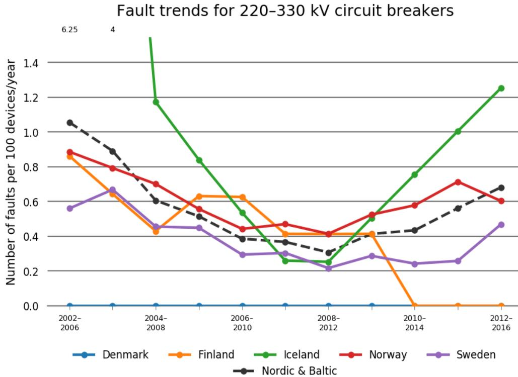
Figure 5.7.2 Fault trends as five-year averages for circuit breakers at the voltage level 220–330 kV in Nordic countries
