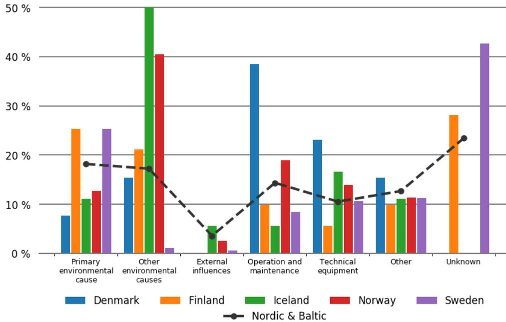
Figure 3.3.3 Percentage distribution of grid disturbances causing ENS per cause in each Nordic country in 2016
