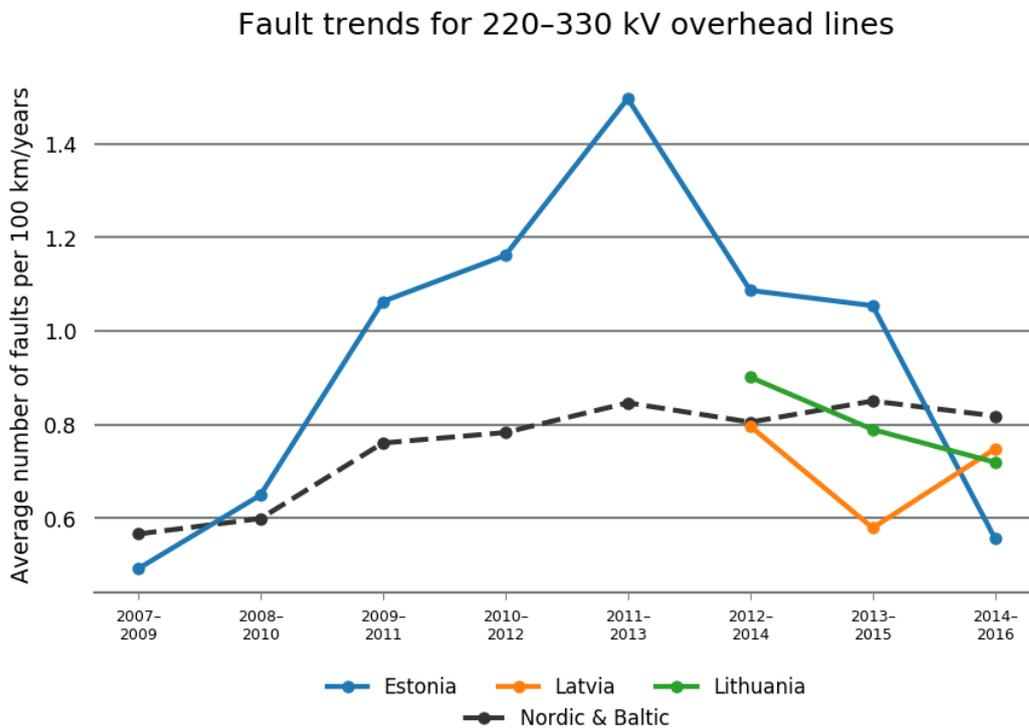
Figure 5.3.12 Fault trends as three-year averages for overhead lines at the voltage level 220–330 kV in each Baltic country. Estonia has reported data since 2007 and Latvia and Lithuania have reported data since 2012.
