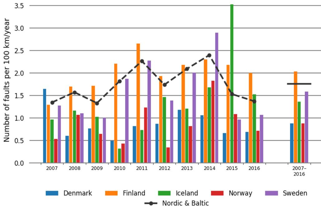
Figure 5.3.6 Annual distribution of line faults for 100–150 kV overhead lines during the period 2007–2016 and the average for 2007–2016 in each Nordic country
