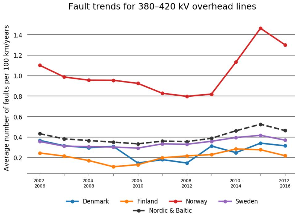
Figure 5.3.10 Fault trends as five-year averages for overhead lines at the voltage level 380–420 kV in Nordic countries
