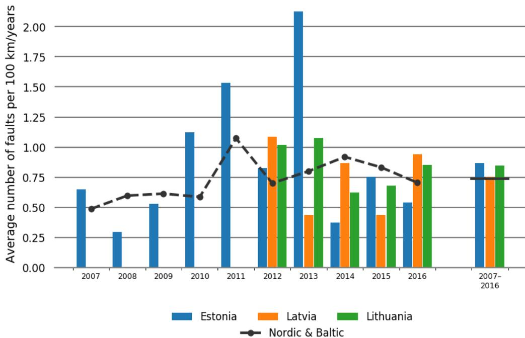
Figure 5.3.3 Annual distribution of faults for 220–330 kV overhead lines during the period 2007–2016 and the average for Estonia during 2007–2016 and for Latvia and Lithuania during 2012–2016
