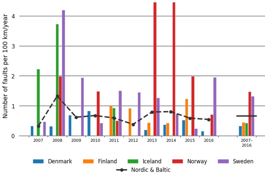
Figure 5.4.1 Annual distribution of 100–150 kV cable faults during the period 2007–2016 and the average for the period 2007–2016 in each Nordic country
