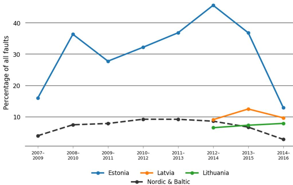
Figure 6.6.11 Fault trends as three-year averages for 220–330 kV operation and maintenance for each Baltic country. Estonia has reported data since 2007 and Latvia and Lithuania have reported data since 2012.
