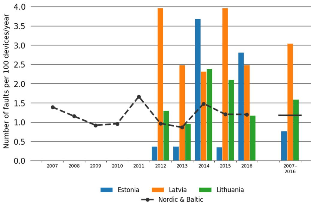
Figure 5.8.5 Annual distribution of 100–150 kV control equipment faults and the average for Estonia during 2007–2016 and for Latvia and Lithuania during 2012–2016
