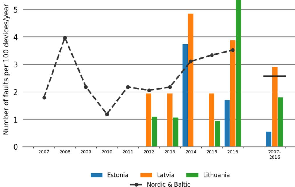
Figure 5.8.3 Annual distribution of 220–330 kV control equipment faults and the average for Estonia during 2007–2016 and for Latvia and Lithuania during 2012–2016
