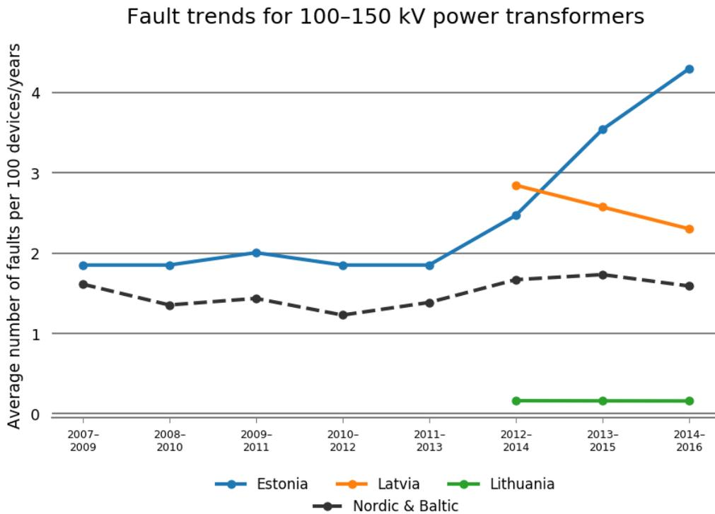
Figure 5.5.10 Fault trends as three-year averages for 100–150 kV power transformers in each Baltic country. Estonia has reported data since 2007 and Latvia and Lithuania have reported data since 2012.
