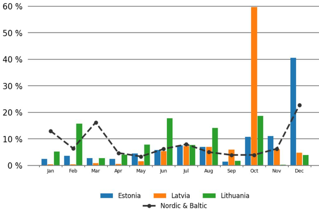
Figure 4.4.4 Average percentage distribution of grid disturbances per month for Estonia during 2007–2016 and for Latvia and Lithuania during 2012–2016
