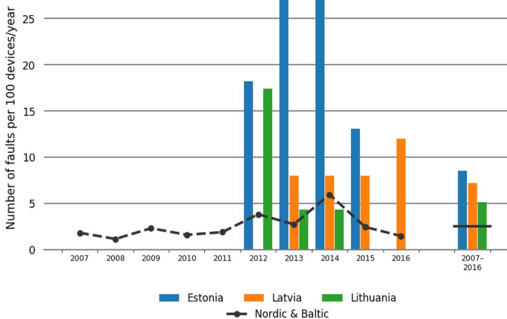
Figure 5.5.3 Annual distribution of faults for 220–330 kV power transformers and the average for Estonia during 2007–2016 and for Latvia and Lithuania during 2012–2016
