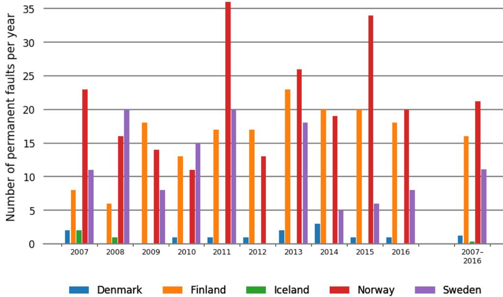
Figure 5.3.8 Annual distribution of permanent faults for 100–150 kV overhead lines during the period 2007–2016 and the average for 2007–2016 in each Nordic country
