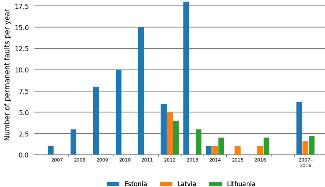
Figure 5.3.5 Annual distribution of permanent faults for 220–330 kV overhead lines during the period 2007–2016 and the average for Estonia during 2007–2016 and for Latvia and Lithuania during 2012–2016
