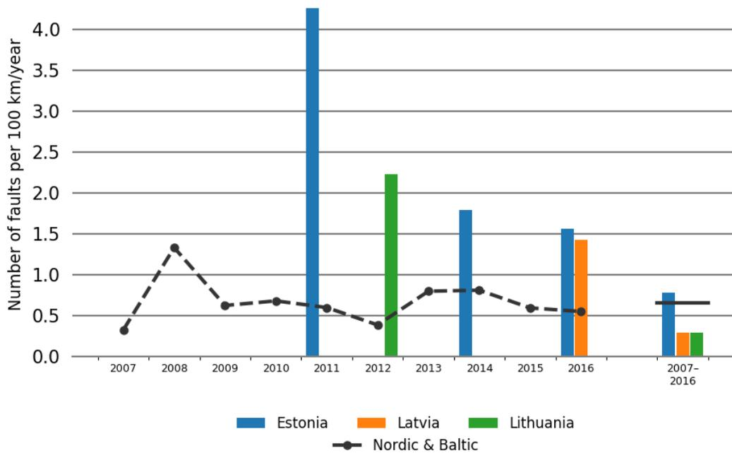
Figure 5.4.2 Annual distribution of 100–150 kV cable faults during the period 2007–2016 and the average for Estonia during 2007–2016 and for Latvia and Lithuania during 2012–2016
