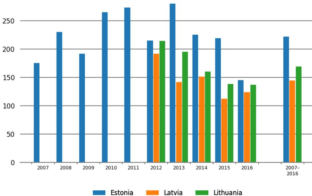
Figure 3.1.2 The annual number of grid disturbances and the average for Estonia for the period 2007–2016 and for Latvia and Lithuania for the period 2012–2016
