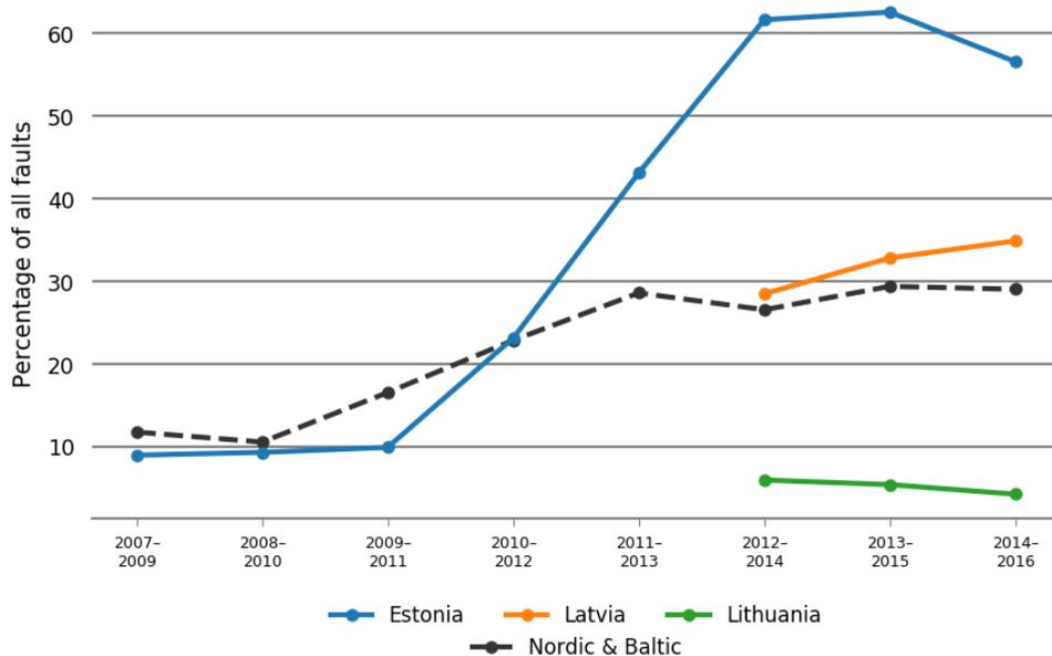
Figure 6.6.2 Fault trends as three-year averages for 100–150 kV other environmental causes for each Baltic country. Estonia has reported data since 2007 and Latvia and Lithuania have reported data since 2012.
