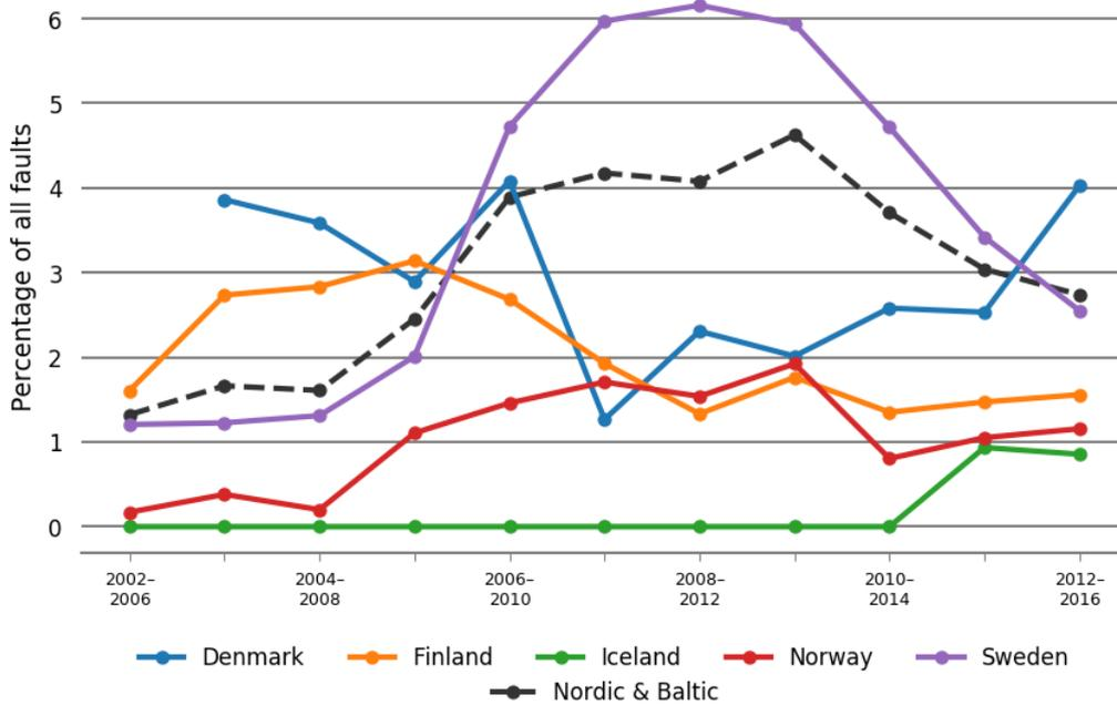
Figure 6.6.8 Fault trends as five-year averages for 100-150 kV operation and maintenance faults for each Nordic country
