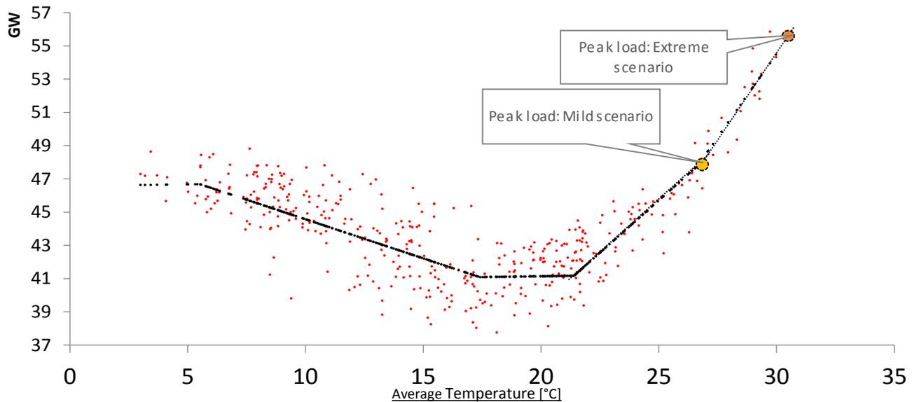
Figure 19: Load-temperature dependency in Italy
