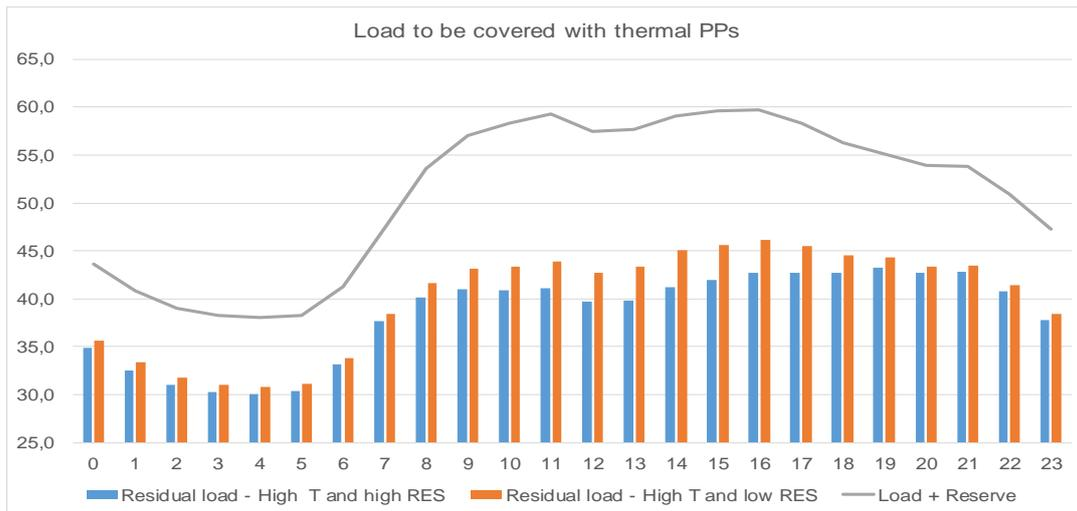
Figure 20: Load curve in Italy and residual load (load to be covered with thermal power plants) profile
