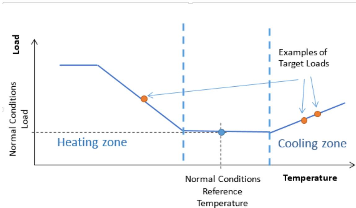
Figure 6: Load-temperature sensitivity.
