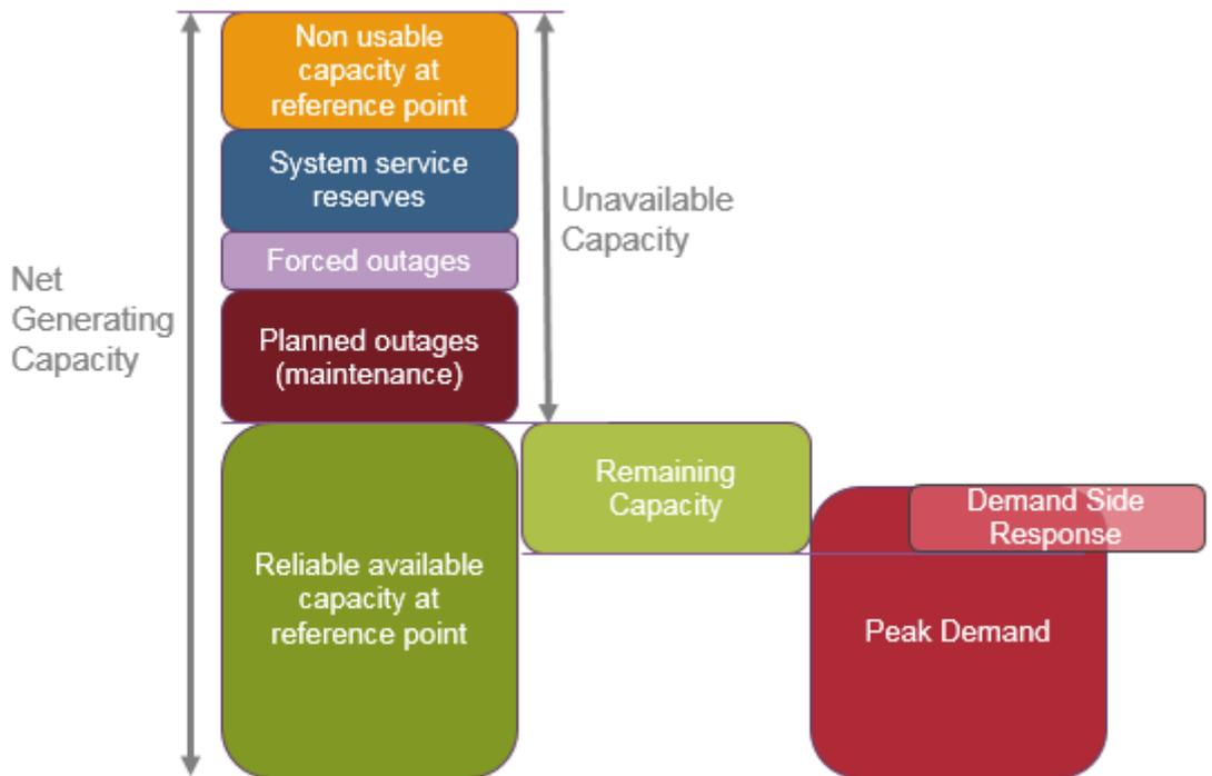
Figure 4: Upward adequacy methodology.
