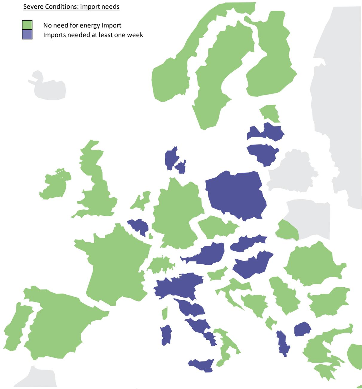
Figure 9: Generation adequacy map at peak time under severe conditions with six nodes in Italy.
