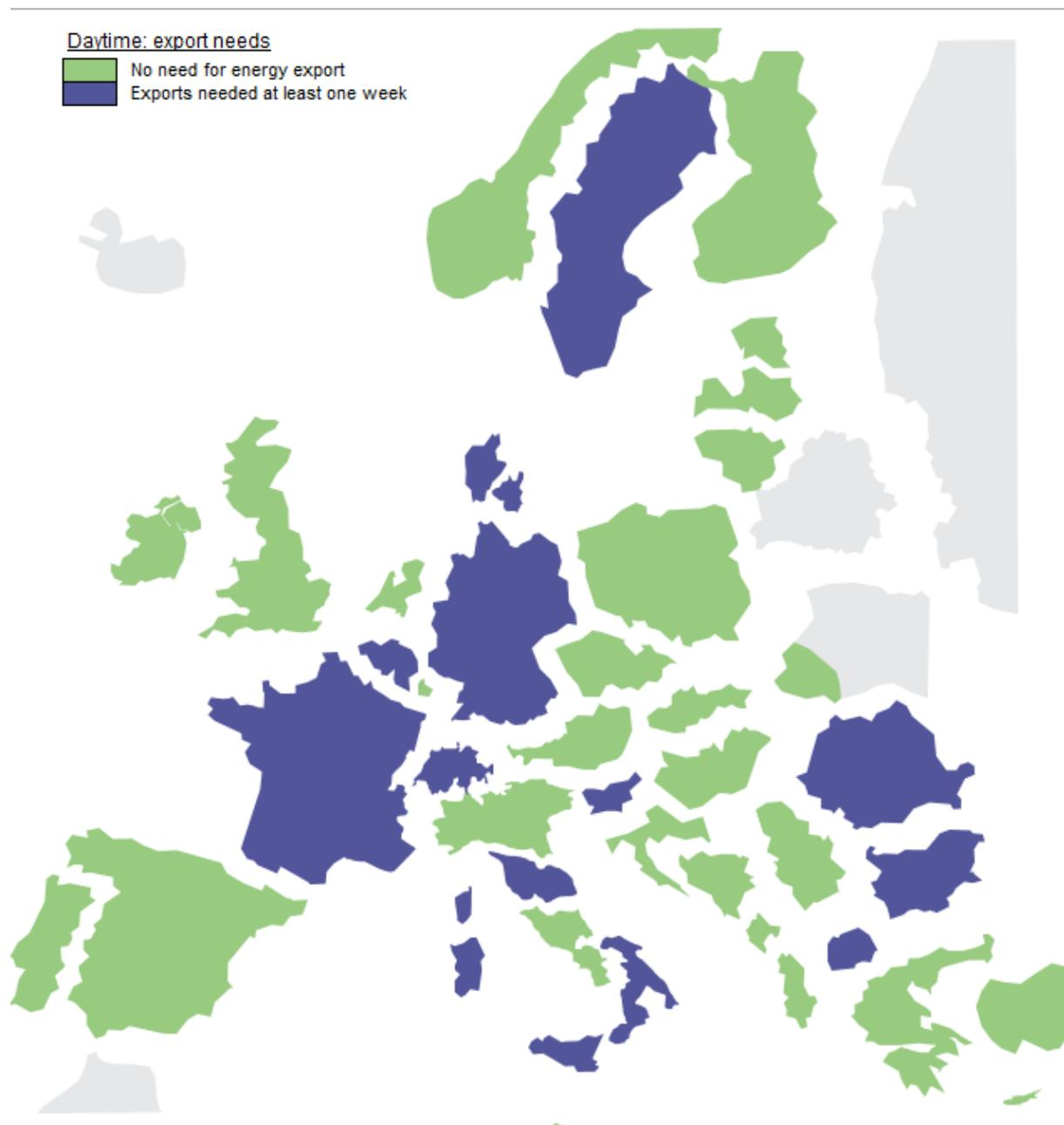
Figure 14: Overview of the export needs for the daytime scenario with six nodes in Italy.
