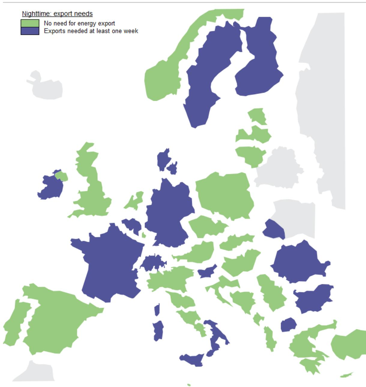
Figure 15: Overview of the export needs for the night-time scenario with six nodes in Italy.
