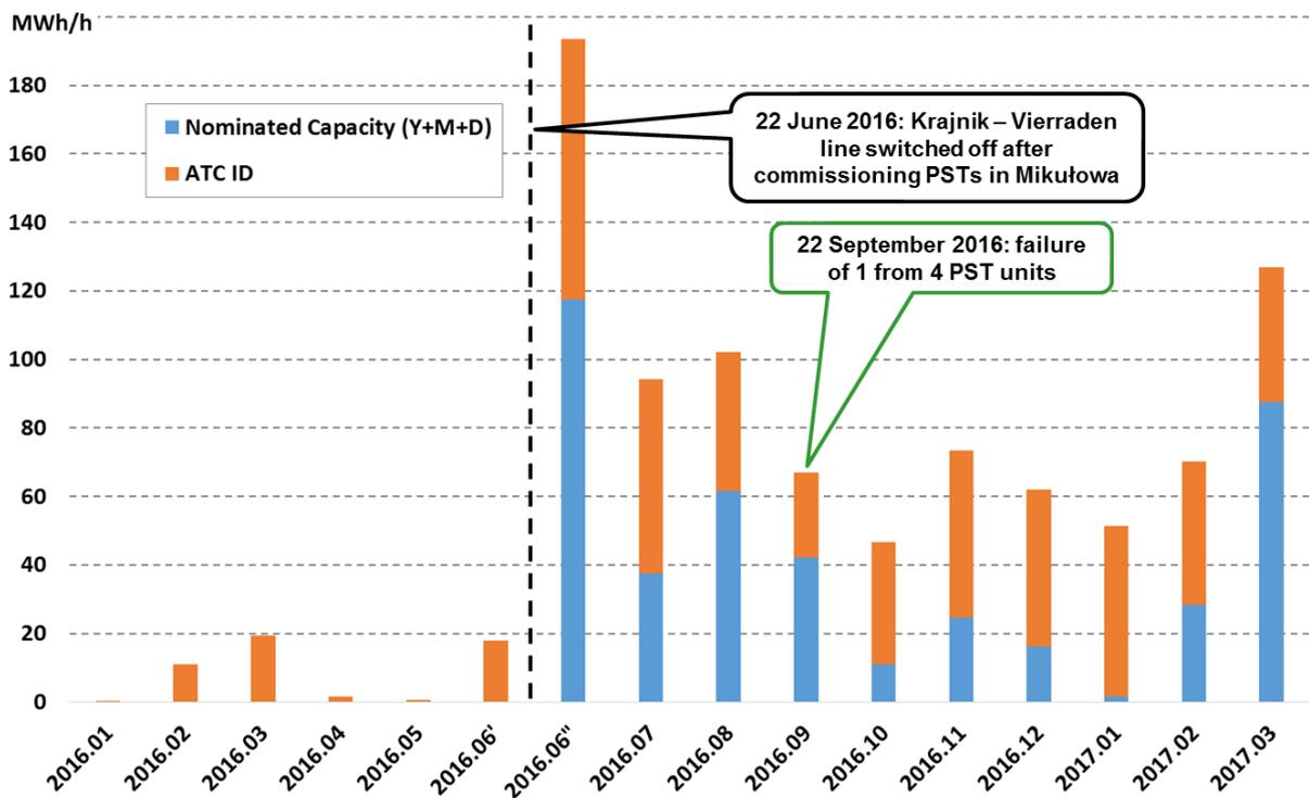
Figure 22: Average monthly import capacity on synchronous profile with DE+CZ+SK before and after reconfiguration on PL-DE border.
