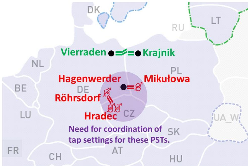
Figure 21: Existing (solid line) and planned / under construction (dotted line) PSTs in the region.
