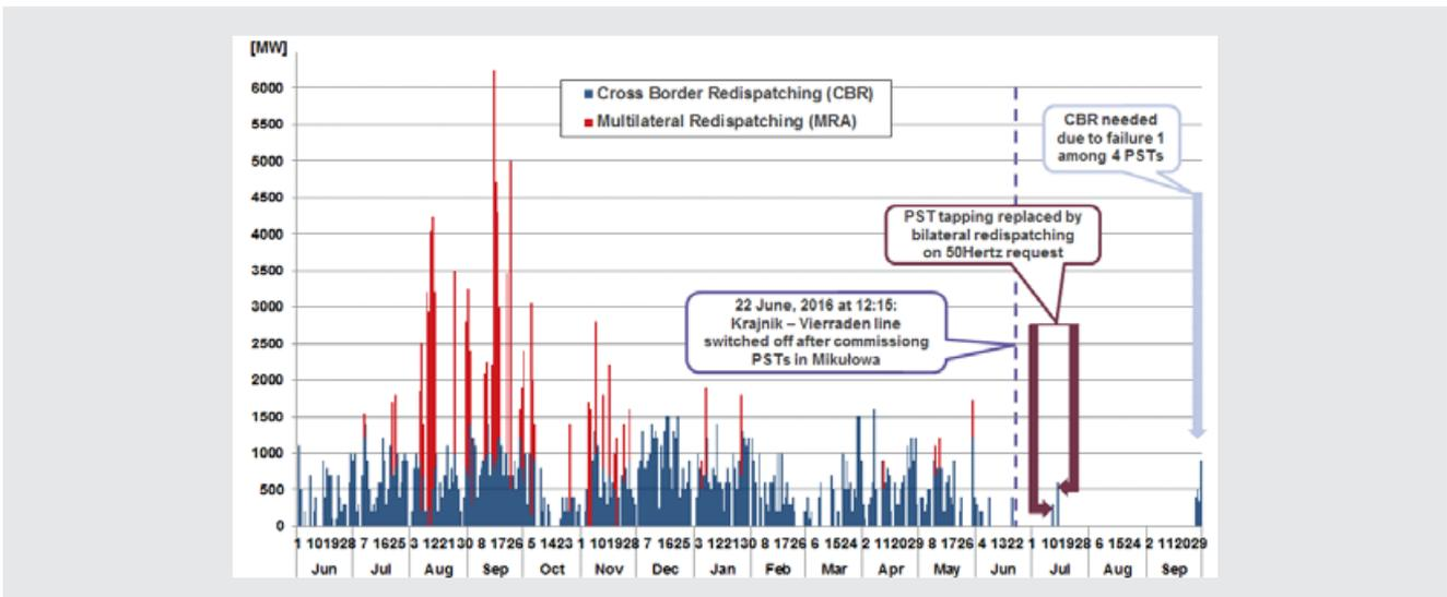
Figure 2: Maximum daily volume of CBR and / or MRA necessary to keep 50Hertz / PSE profile in N-1 secure state.
