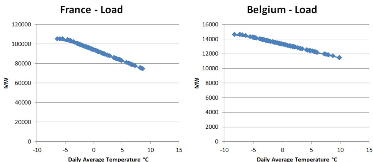
Figure 11 - Simulated temperature dependence of load for France (left) and Belgium (right)
