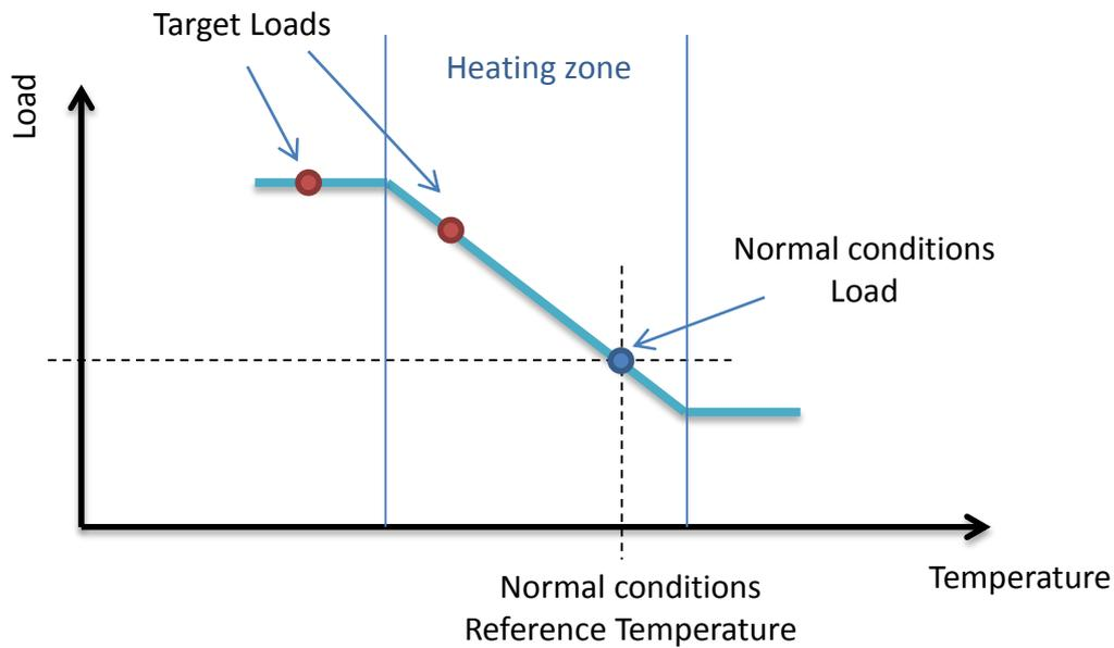
*Figure 1 – Load temperature sensitivity*
