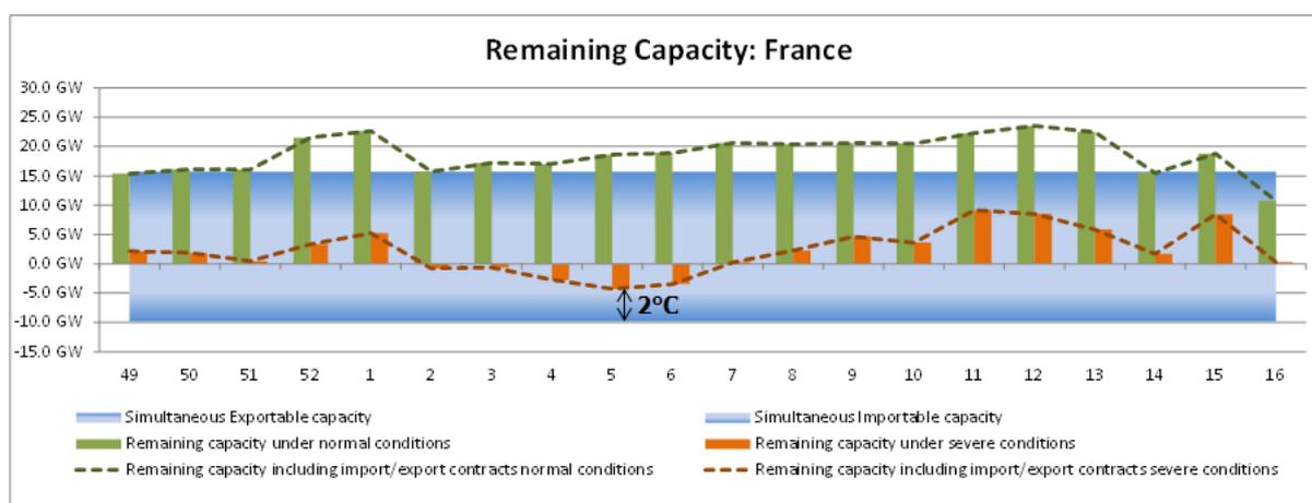
Figure 6 - Illustration of temperature sensitivity of margins (France)
