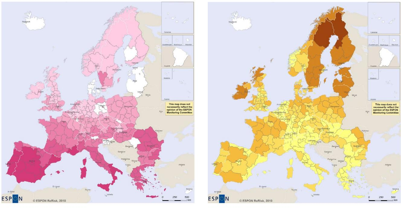
Figure 7: PV and wind power potential in Europe
