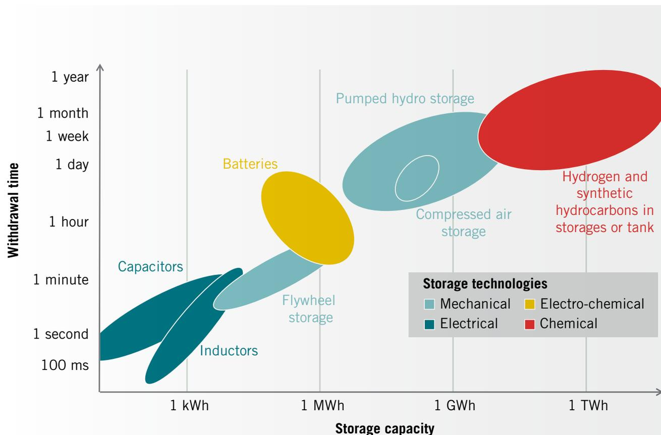
Figure 12: Differences in storage capacity and withdrawal time for various storage methods
