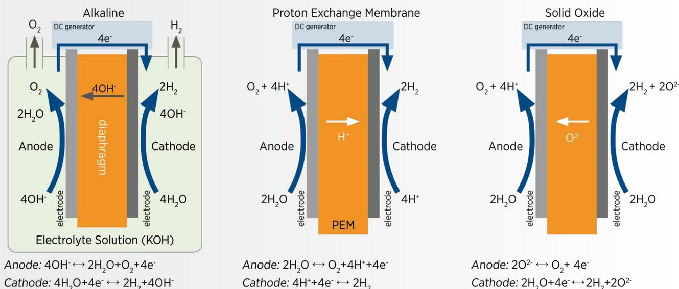
Figure 1: Illustration of the three main types of electrolysers
