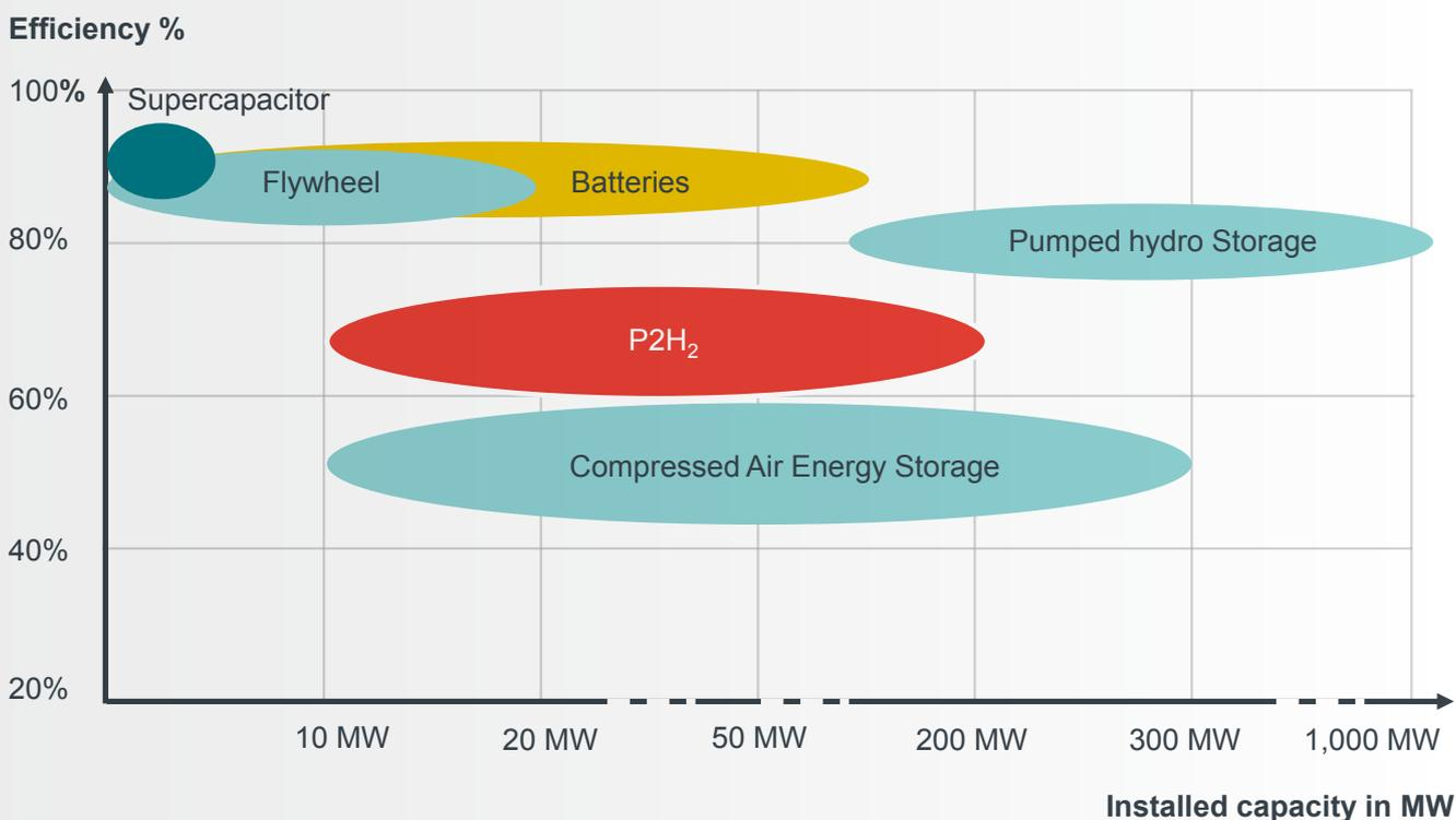
Figure 13: Efficiency and average installed capacity (per unit) for each technology in the EU (not accounting for reverse operation)
