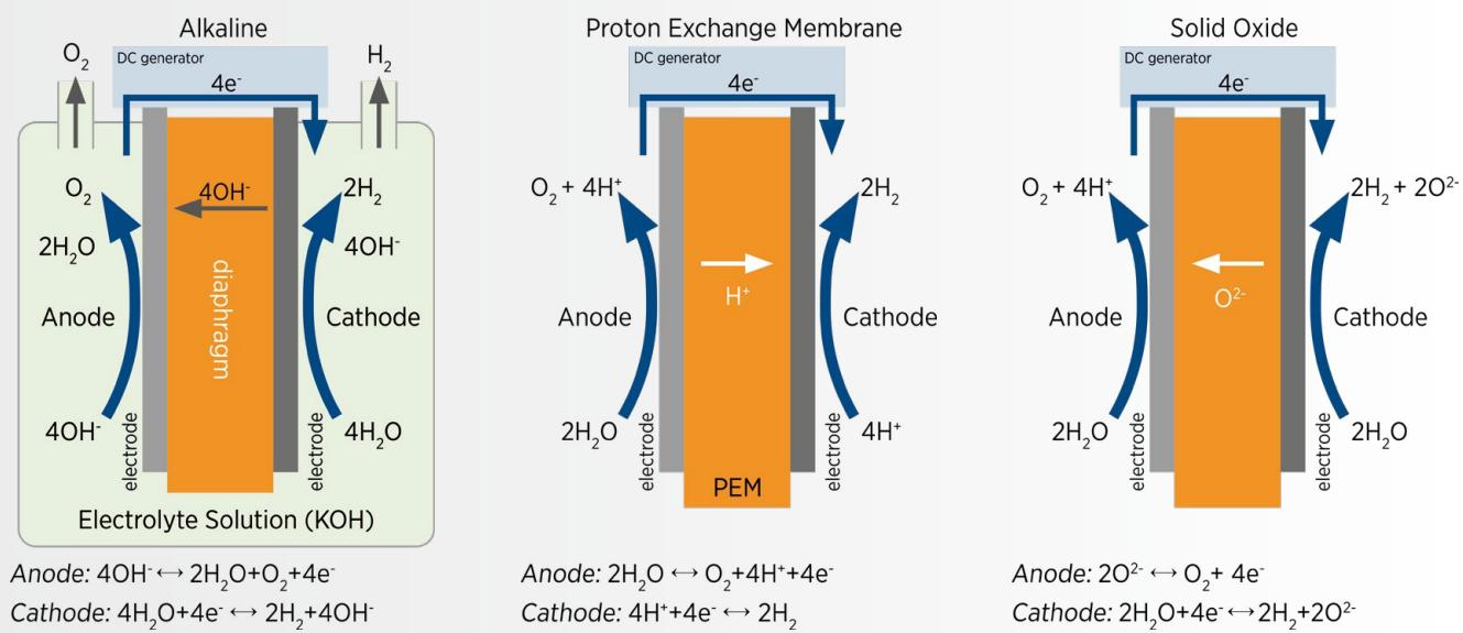
Figure 1: Illustration of the three main types of electrolyzers
