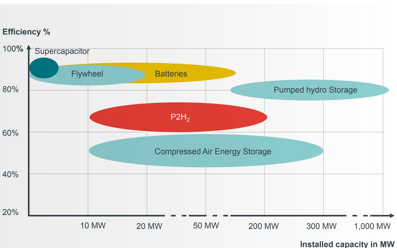
Figure 13: Efficiency and average installed capacity (per unit) for each technology in the EU (not accounting for reverse operation)
