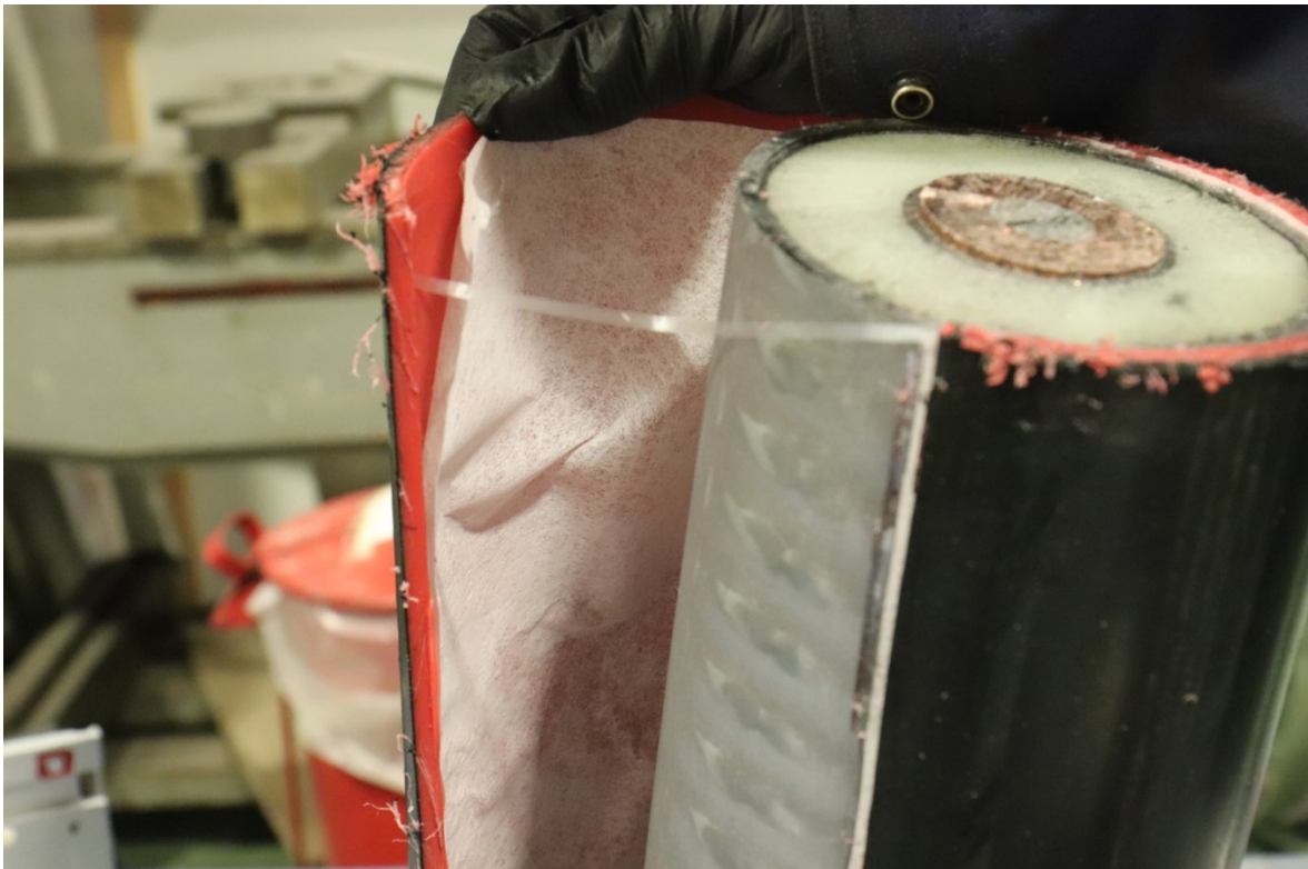
Figure 7-31: Sample 5 after longitudinal cut in PE sheath. A layer of paper was present between the PE and the lead layer.
