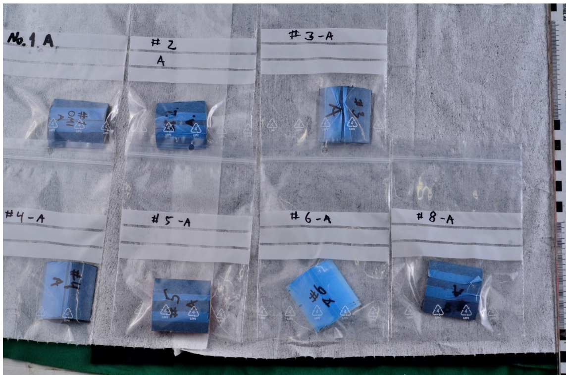
Figure 7-39 Samples extracted from polymer sheath masked and section to size of approx. 50 x 50 mm.
