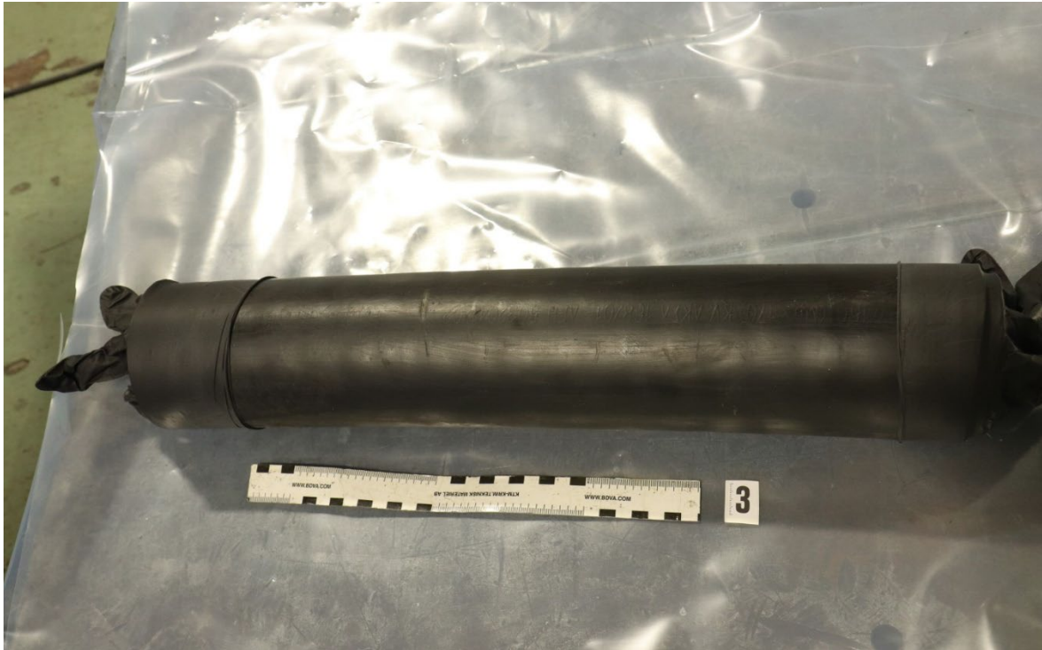
Figure 7-19: Sample 3 as received and cut to length, and with protection on the cut surfaces (nitrile gloves).
