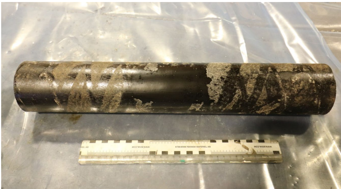
Figure 7-25: Sample 4 PE sheath overview.
