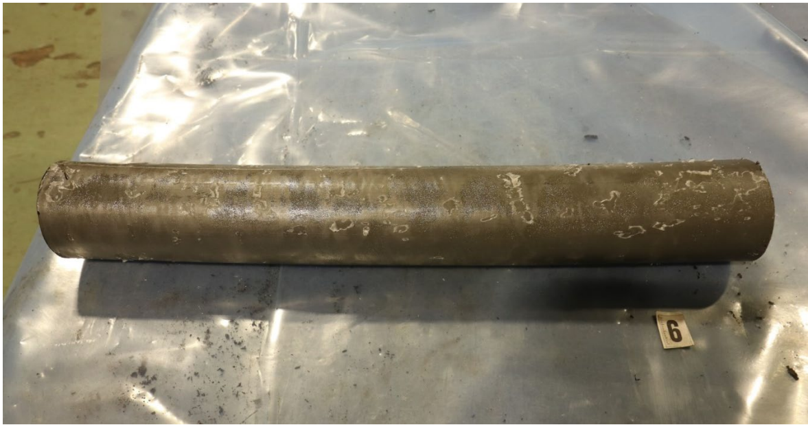
Figure 7-35: Sample 6 after removal of PE/PP sheath – lead sheath revealed.
