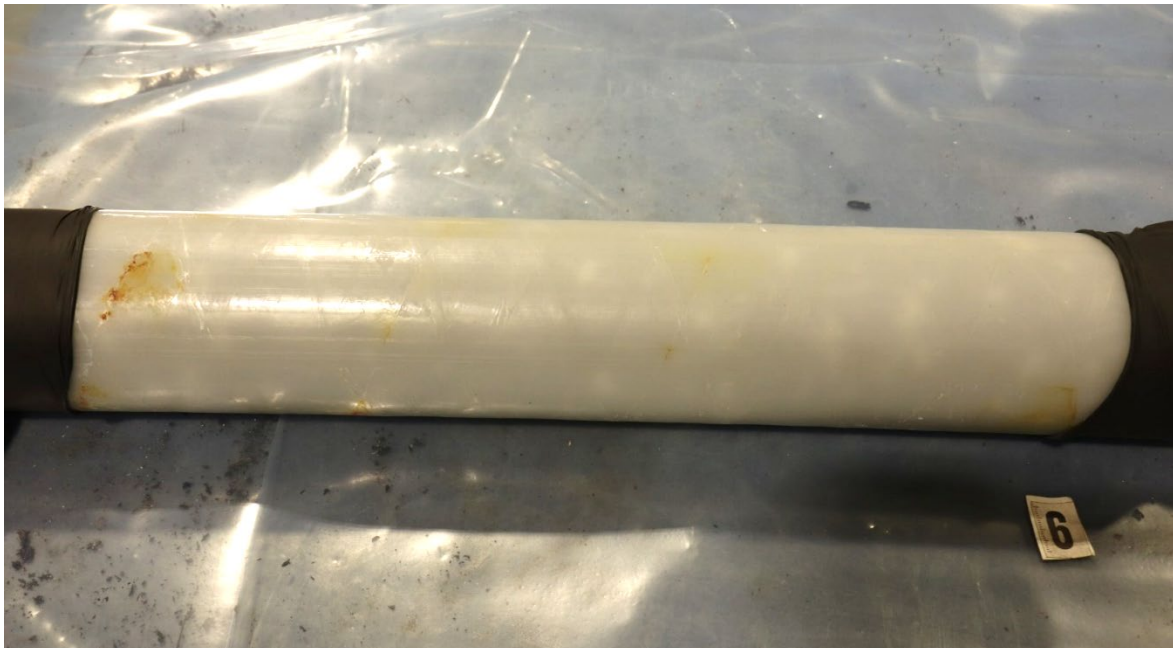
Figure 7-34: Sample 6 overview of PE/PP sheath, and with protection on the cut surfaces (nitrile gloves).
