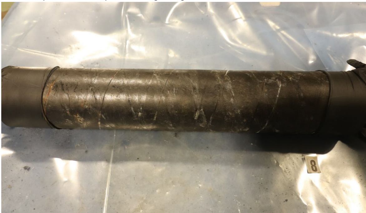
Figure 7-37: Sample 8 overview of PE/PP sheath, and with protection on the cut surfaces (nitrile gloves).
