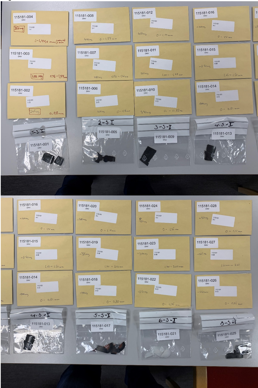
Figure 3-12 Samples for ICP testing. Paper bags are samples from microtome cutting and samples in plastic bag is shavings taken during dissection.
