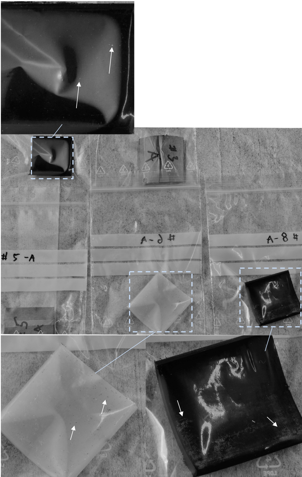
Figure 7-40 Images illustrating observations on the inner surface of sample No. 2, 6 and 8. Sample 2 and 6 was not possible to clean on polymer sheath inner surface (facing the lead) with ethanol due to a sticky residue. Sample No. 8 had staining on inner surface facing the lead not removed by cleaning. Arrows indicate particles/ residue on inner surface and staining.
