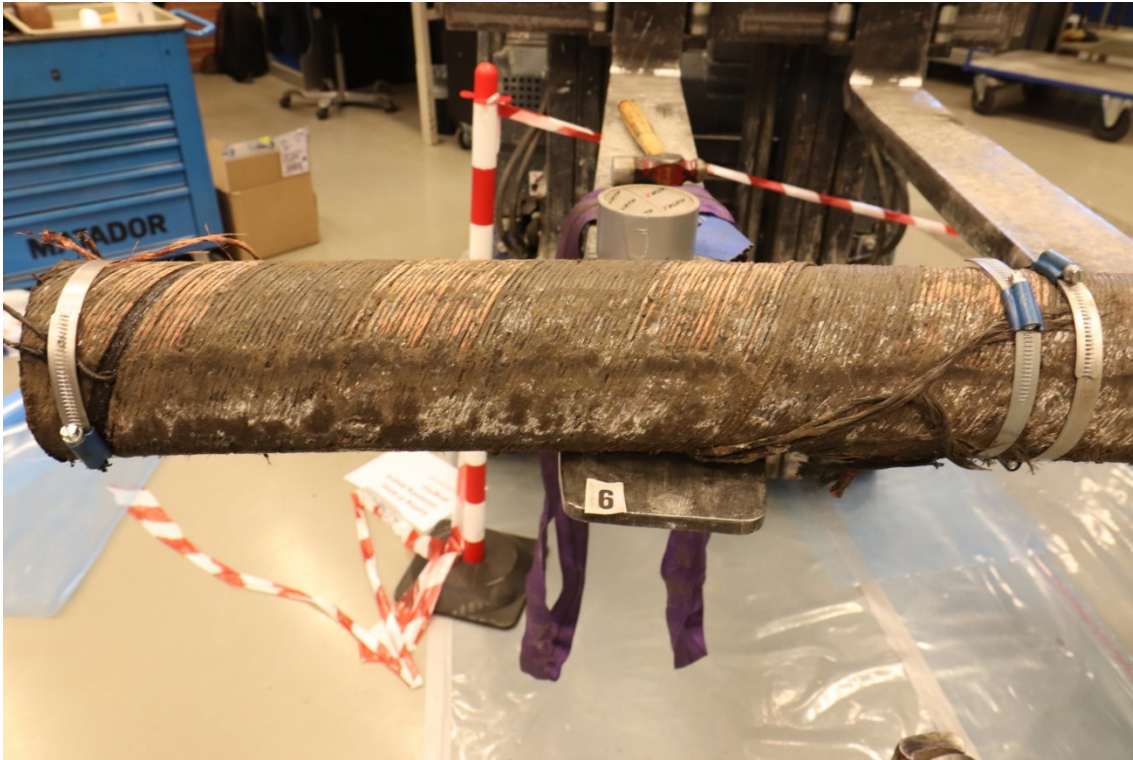
Figure 7-33 Sample No. 6 as received prior to cutting to length
