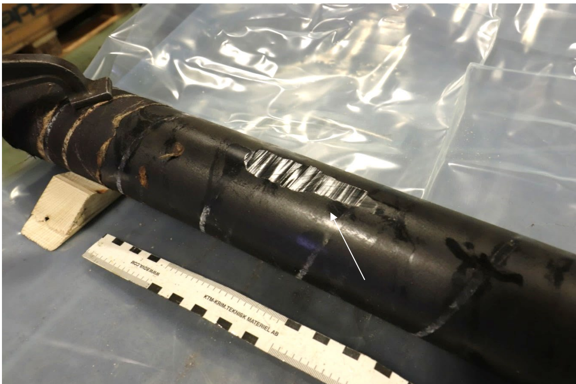
Figure 7-10: Sample 1 PE sheath after extraction of shaving samples.
