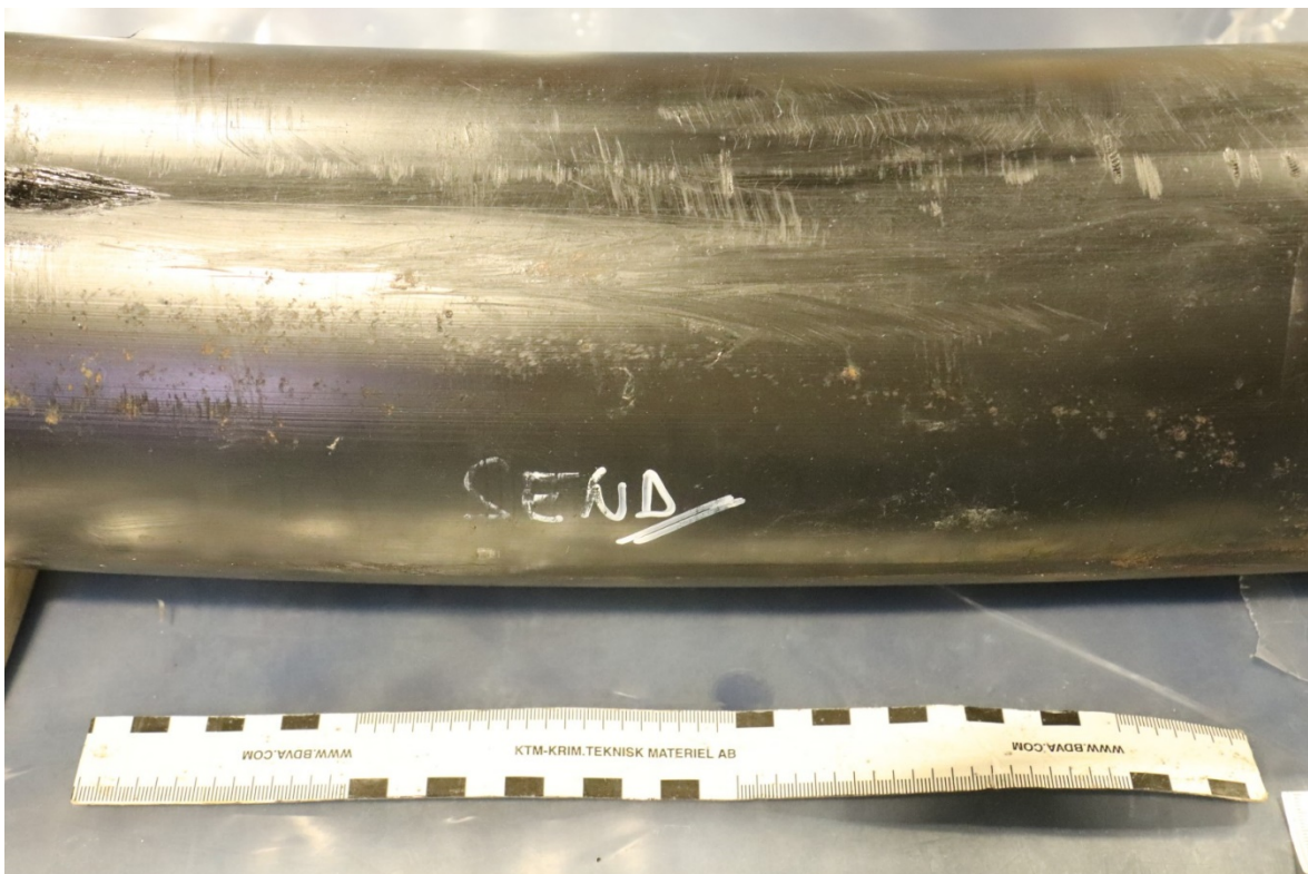
Figure 7-29: Sample 5 close-up of the outer surface of the PE sheath.
