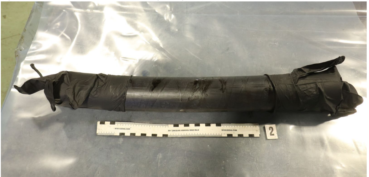
Figure 7-14: Sample 2 overview of polymer sheath and with protection on the cut surfaces (nitrile gloves).
