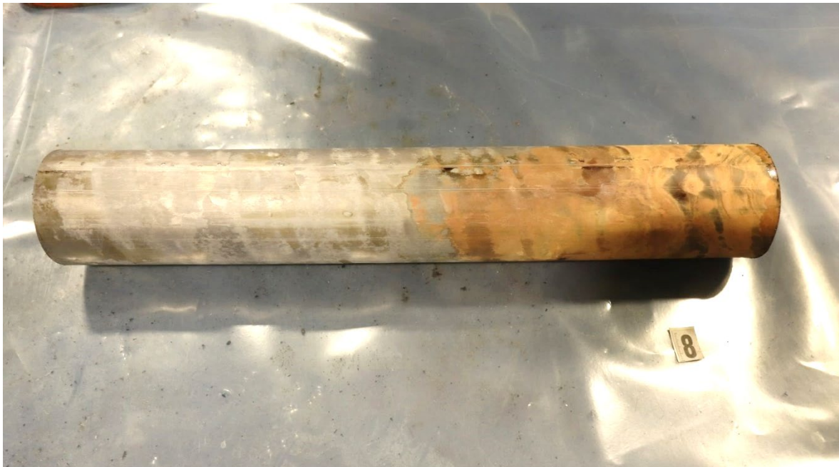
Figure 7-38: Sample 8 after removal of PE sheath – lead sheath revealed. Discoloration of lead sheath.
