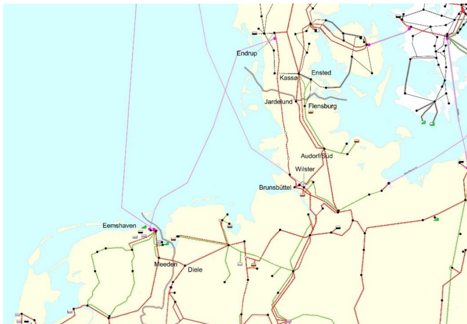
Figure 5: Gridmap of the border between DK1 and NL – the Cobra cable
