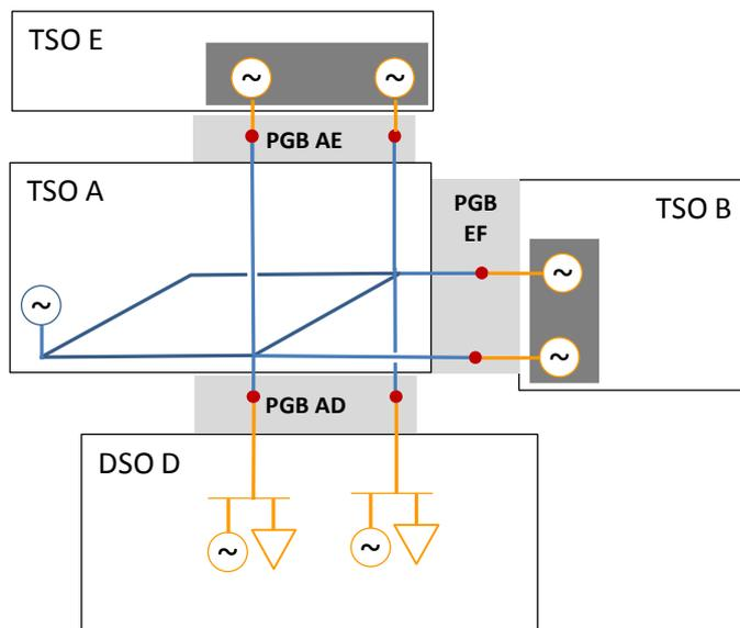
Figure 7 TSO A DACF Network model
