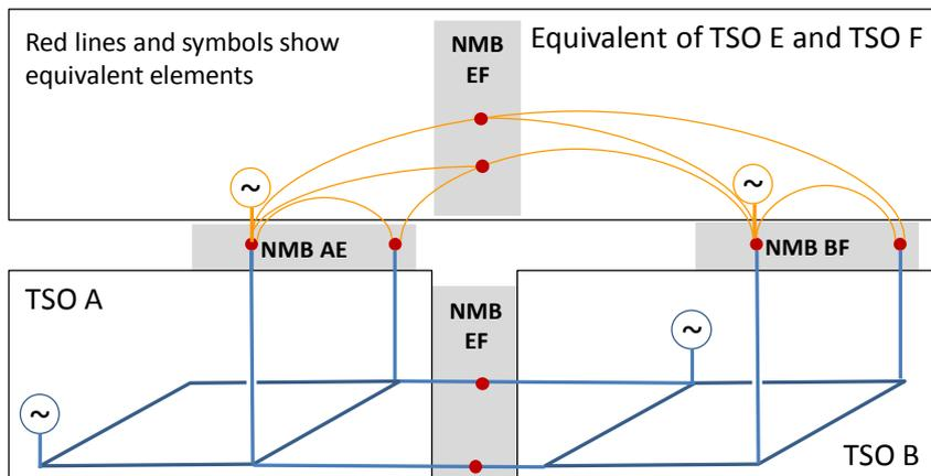
Figure 5 Equivalent from Fully Reduced TSO E and TSO F Networks
