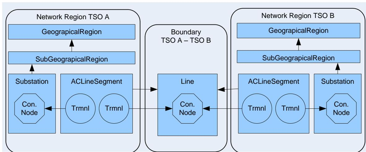
Figure 3 Detailed CIM data diagram for the tie line between tso a and tso b
