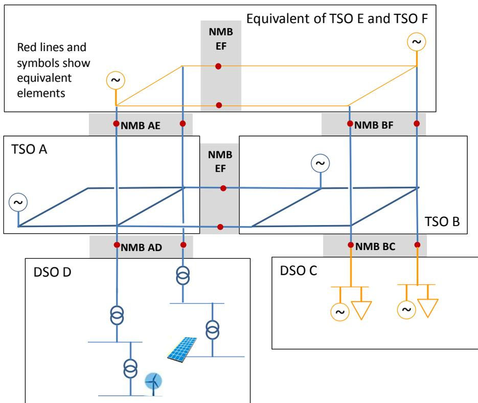
Figure 6 Power grid model as seen from TSO A
