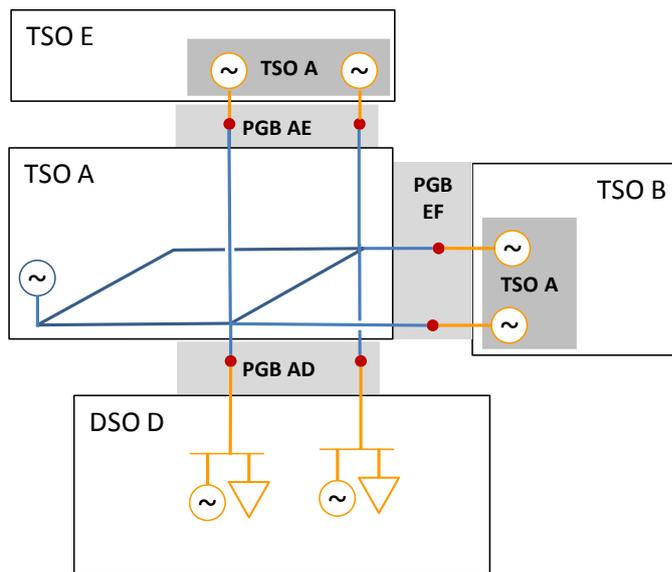
Figure 4 Example where TSO A has replaced TSO B and TSO E with Network Edges
