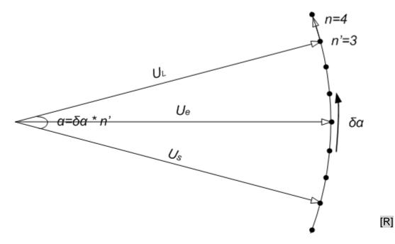
Principle of a symmetrical PST device with constant impedance or voltage:
