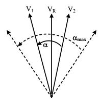
$$X_{n} = X_{\min} + \left(X_{\max} - X_{\min}\right) \left(\frac{\sin(\alpha_{n}/2)}{\sin(\alpha_{\max}/2)}\right)^{2}$$
