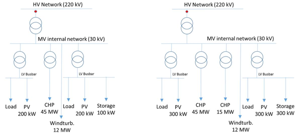
Mixed sites connected at HV network via internal (= private) MV grid
